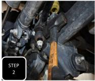
**Step 2** Unbolt the nut attaching the track bar to the axle and then brake the joint loose by hitting the side of the axle mount with a hammer. **NOTE: NEVER HIT THE ROD END ON THE THREADS.**
