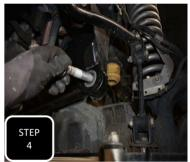
**Step 4** Loosely attach the new adjustable trac bar using the factory bolt at the frame and the provided nut at the axle then torque both to factory specs.
