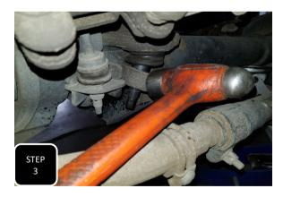
**Step 3** Remove the nut from the ball joint where the trac bar attaches at the axle and hit the side of the trac bar, right at the joint, with a hammer to break it loose.
