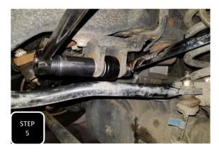
**Step 5** Re-install the wheels and tires, lower the truck back to ride height, and tighten the frame side of the trac bar. Torque to factory specs.
