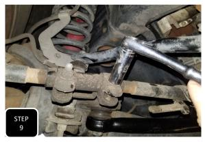
**Step 9** Loosen both of the clamps on the drag link adjuster and spin the collar until the steering wheel is straight and tighten both clamps back down. Next, go drive the truck to make sure the wheel is straight then make further adjustments as needed.
