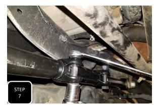
**Step 7** Adjust the collar on the trac bar in the direction needed until your measurements on both sides read the same. Then tighten down the clamps on the trac bar.
