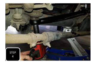
**Step 4** Loosely attach the new, adjustable trac bar using the factory hardware. **NOTE: THE BALL JOINT AT THE AXLE CAN BE FULLY TIGHTENED, BUT DO NOT TIGHTEN THE BUSHING AT THE FRAME UNTIL THE TRUCK IS AT RIDE HEIGHT.**
