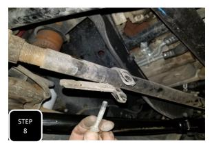
**Step 8** The steering wheel will now need to be straightened so start by unbolting and removing the safety tabe the for the drag link and sliding it out of the way.
