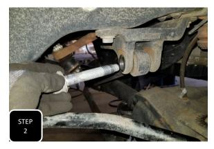
**Step 2** Unbolt the trac bar from the mount on the frame, remove the bolt, and lower separate.
