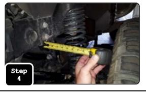
**Step 5:** Loosen the adjustment collar clamps and slide them out of the way. now twist the adjustment collar out and keep comparing your measurements until you measure the same distance from frame to tire on both sides.
