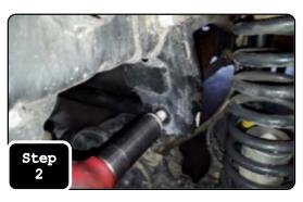
**Step 3:** Install the new Maxtrac adjustable trac bar with the U shape over the differential using the factory bolts. Adjust the height of the body as necessary so that the bolts are easy to install. let the jack all the way down, jounce the front bumper a few times to settle the suspension and then tighten both bolts.
