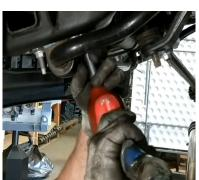
Unbolt the sway bar from the sway bar end links on both sides of the vehicle. Save the hardware for reuse.
