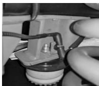
On the driver side, attach the vacuum line to the new bump stop drop bracket.
