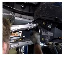
Install the 4 link arms at this time. Start with the upper arm then the lower arm. Use the provided 9/16-12x4 & x 5" bolts for the links at the hangers, Then use the provided M18 X 140 bolts and steel sleeves at the axle to mount the arms. Next, insert the clamp bolts and tighten.
