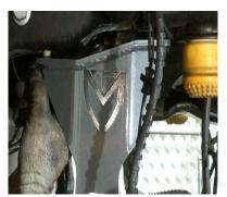
Install track bar drop bracket using provided 3 way bolt bracket. Use thread locker on the bolts. Torque OE the bolts to 129 ft. lbs.
