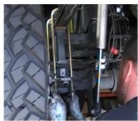
Install the supplied lift block Make sure the pin fits into the hole on the spring perch. Use your floor jack to raise the axle to the spring making sure the pin on the factory leaf spring assembly fits into the hole on the lift block. Secure the assembly with the hi-nuts washers supplied. Do not torque the hi-nuts at this time.
