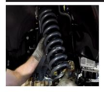
Using the factory isolators install the supplied front coil springs into the spring buckets and raise the axle into place. Make sure the coil spring seats properly on the lower spring perch.
