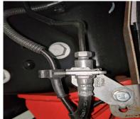
Install the driver and passenger side maxtrac brake line extension brackets to the side of the coil buckets using the provided 8mm hardware. Once this is done carefully unbend the metal brake lines until they align with new mounting holes that are attached at the bottom of the maxtrac brake line brackets.
