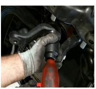
Reinstall the Pitman arm retaining nut to the sector shaft and torque to 350 ft./lbs.
