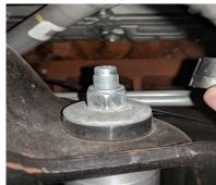
Install the new front shocks at this time using the factory hardware.
