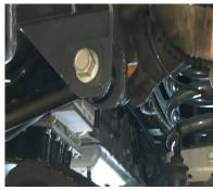
Reinstall the track bar into the Maxtrac track bar bracket using the OE bolt and adjustable cam plate. Torque to 406 ft. lbs.
