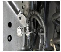
Unbolt the brake front brake lines from the frame.
