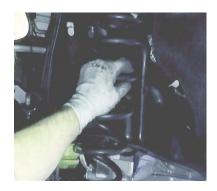
Lower the front axle enough to remove the coil springs from the front spring pockets. Save the factory isolators for re- use.
