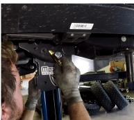
Insert the link arm bracket inside of the original radius arm pocket. The brackets are side specific and will display the Maxtrac logo outwards. While holding the bracket up, line the two holes up and insert the provided M18x130 bolt into the original radius arm bolt hole. Next, install the reduction spacers into the smaller holes just in front of the M18 bolt. Do not install the bolt until the arm is installed
