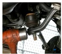
Remove the cotter pin and nut from the drag link, at the pitman arm. Save the nut for re-installation. Use a tie rod separator to separate drag link from Pitman arm.
