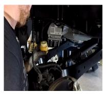
Remove the factory front bump stops from the bump stop mounting cups. Pliers and a back and forth rocking motion will assist in removal of the bump stops.
