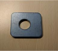
Place the cam on the front side of the trac bar bracket while installing the trac bar and hardware. The Cam will center the axle under the vehicle.
