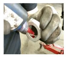
Install new pitman arm on sector shaft. Lock-tite the sector shaft threads to ensure a proper torque reading. Install Pitman arm retaining nut and tighten until snug.
