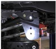
Place a jack under the pinion or radius arm. On both sides remove the rear bolts holding the radius arms to the frame of the vehicle.
