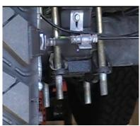
Support the rear axle with a floor jack and remove the U-bolts on the driver side. Slightly loosen the U-bolts on the passenger side.
