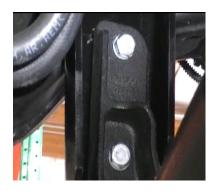
If the vehicle is equipped with a factory steering stabilizer, unbolt it from the frame mount on the passenger side.
