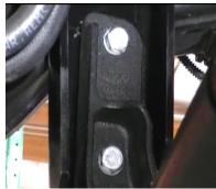
Re-install the factory steering stabilizer bracket to the new drop down bracket. Next, re-install the steering stabilizer back on the OE bracket
