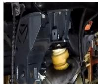
Reinstall the previously removed factory bump stops into the mounting cup on the new bump stop drops.
