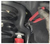
On the driver side, unclip the axle vent line from inside the frame.
