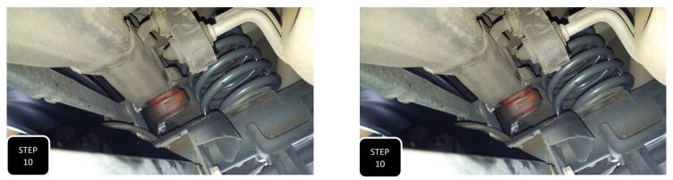
Step 10 Once cut, re-install the bump stops and there should be about 1-2" of gap depending on the amount of drop.
