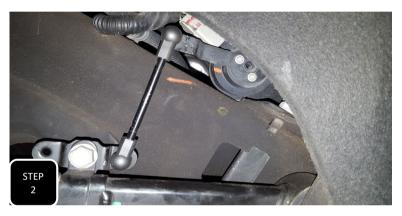
**Step 2** Remove the factory sensor rods attached towards the front of upper link arms by using a prefered prying tool to pop the plastic rod end off of the attached metal ball.
