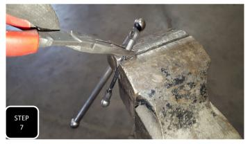
**Step 7** Clamp the factory sensor rod in a vise allowing room to grab between the rod and rod end with needle nose pliars. Using the surface of the vise as a leverage point, pry upward to pop the plastic rod end off of the factory rod. **NOTE: USE YOUR OTHER HAND AS A BLOCKER SO THAT THE PLASTIC ROD END DOES NOT GO FLYING AND GET LOST.**
