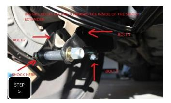
**Step 5** Install the provided shock extenders over the factory shock mounts on the axle. Use the provided 1/2" bolts through the original shock mount holes, from the outside facing in along with the provided lock washers and jam nuts. Next, us the longer 1/2" bolt to attach the back of the extender up through the bottom of the factory mount and tighten
