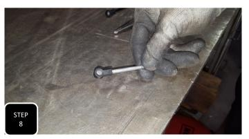
2" drop, the rod should measure 2 15/16" from eye to eye with the rod ends screwed on. (2 3/8" rod only length)
