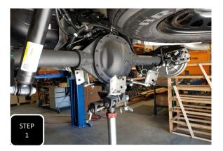
**Step 1** Jack up the rear of the vehicle and support under the frame rails with jack stands. Leave an adjustable jack under the diff for height adjustment.
