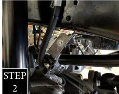
STEP 2: Unbolt the front brake line brackets at the frame and stretch the brake line down a little bit so that the line does not get damaged when installing the coils.
