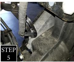
STEP 5: Before lowering the axle, release the two guide clips holding the wiring for the front diff disconnect so that the wire does not get stretched out and damaged.
