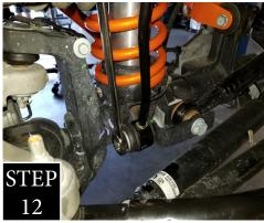
STEP 12: Using the stock hardware, attach the rear sway bar end links to the front and tighten.
