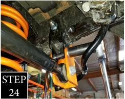
STEP 24: Attach the trac bar to the new bracket using the factory bolt. Tighten the two provided bolts, but only loosely snug up the bolt going through the trac bar. It will get tightened when the truck is back on the ground. (Tightening the trac bar while the suspension is drooped out will cause premature bushing failure and un-safe suspension movement)
