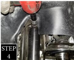
STEP 4: Jack up the adjustable jack enough to take load off of the shocks, then unbolt both shocks at both ends and remove.
