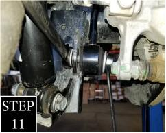
STEP 11: Your factory rear sway bar end links will now be used in the front, so proceed to the rear of the truck and remove the factory sway bar end links.
