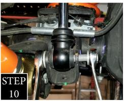
STEP 10: Loosely attach your new shock to the frame using the factory bolt. Jack the axle up enough to attach the lower end of the shock to the axle using the factory bolt and tighten both bolts.
