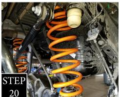
STEP 19: Lower the axle down and remove both rear coil springs.
