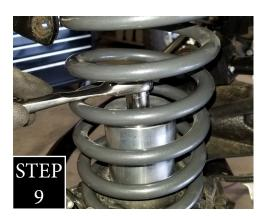
STEP 9: Using the provided 7/16-14 x 2 ½" bolt, attach the bump stop extension to the axle and tighten. (Placing a deep socket into the bump stop extension and then attaching the ratchet to the socket will ease the process of getting the tools between the coils.
