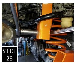
STEP 28: Install the wheels and tires, remove the jack stands and lower the truck to the ground. Jump on the bumper a few times to settle the rear suspension and then tighten the trac bar.
