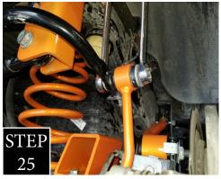
STEP 25: Install the new rear sway bar end links using the factory bolts at the sway bar and the provided M12-1.75X65 bolts, nuts, and washer at the axle. (The sway bar end links should be oriented to where they swoop inward at the axle)
