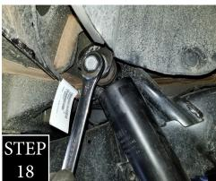
STEP 18: Unbolt both rear shocks at both ends and remove.
