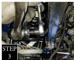
STEP 3: Unbolt the sway bar end links at both ends and remove the links.
