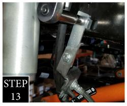
STEP 13: Install the brake line extensions using the factory hardware at the frame and the provided ¼-20 x ¾" bolt, nut, and washers where the two brackets connect. The bent tab on the provided bracket should face outward and not line up with anything. The bent tab on the factory bracket needs to be rotated so that it contacts the new bracket, then tighten.
