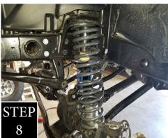
STEP 8: While holding the billet aluminium bump stop extension inside the new coil, install the new coil onto the truck. (The part number should be right side up)
