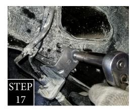
STEP 17: Unbolt the rear brake line brackets at the frame and stretch the hardline down a little bit so that the brake lines don't get stretched out when installing the coils.
