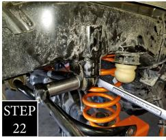
STEP 21: Attach the new bump stop extension to factory striker plate on the axle using the provided 3/8-16 x 1" bolts, nuts and washers. (En-sure that the bump stop extension is installed with the angle cut leaning forward.
