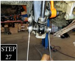
STEP 27: Loosely attach your new shock to the frame using the factory bolt. Jack the axle up enough to attach the lower end of the shock to the axle using the factory bolt and tighten both bolts.
