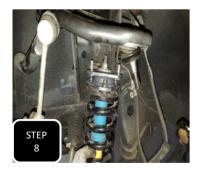
**Step 8** Re-install the strut assembly back into the truck and loosely attach the hardware at the top and bottom.
