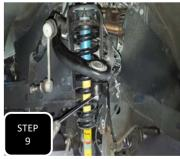
**Step 9** Place a floor jack under the lower control arm and jack up to compress the coil. Now re-attach the upper control arm to the spindle, tighten the castle nut, and reinstall the factory clip.
