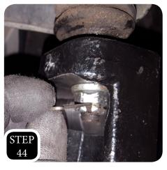
**STEP 44:** Re-install the cotter clip into the castle nut of the upper control arm.
