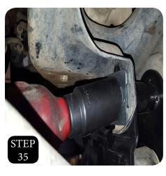
**STEP 35:** Now that all of the diff mounts have been attached and the LCA's are loosely installed, tighten down all diff mounts at the subframes and then tighten down all 4 subframe bolts where they attach to the frame.
