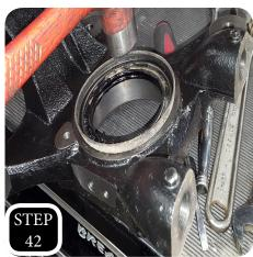
**STEP 42:** Gently pop the factory dust seal out of the back of the factory knuckle and install it into the back of the Max Trac steering knuckle.
