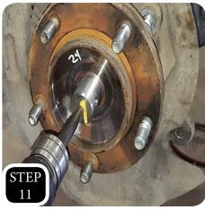
STEP 11: Unbolt the four wheel bearing bolts and remove. If you have trouble removing the axle, use an air hammer at the end of the axle to push it through.
