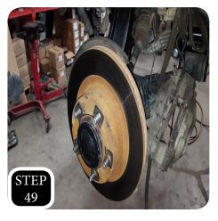
**STEP 49:** Re-install the brake rotor.
