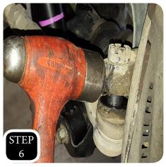
**STEP 6:** Remove the tie rod cotter pin, remove the nut, and separate by hitting the side of the steering arm with a hammer.
