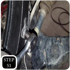
**STEP 51:** Attach the brake line guide bracket to the back side of the neck of the steering knuckle, just under the ABS guide bracket, using the factory bolt.
