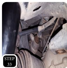
STEP 33: Insert the provided vacuum connecter into the provided breather line extension. Next attach one end to the breather hose and the other end to the diff.
