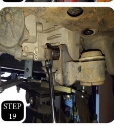
**STEP 19:** Lower the diff slightly and unbolt both the pass side mount and the front mount from the diff.
