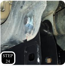
**STEP 24:** Loosely install the rear subframe with the side mounting tabs facing forward using the provided M18-2.5 x 150 bolts, small holed square washers, and nuts.
