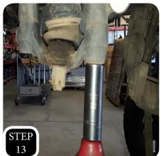
**STEP 13:** Break the upper ball joint loose by hitting the side of the upper ball joint boss with a hammer, then loosen both lower bolts and remove the steering knuckle.
