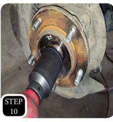
**STEP 10:** Remove the castle retainer and then the axle nut using a 38MM, 12 point socket.
