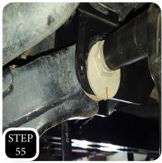
**STEP 55:** Snug up, but do not tighten all 4 alignment cam bolts. They will get tightened when the truck is back on the ground.
