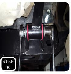
STEP 30: Loosely attach the front diff mount and the drivers rear diff mount to the subframes using the provided 9/16-12 x 4.5" bolts, nuts and washers.
