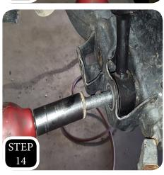
**STEP 14:** Remove all 4 upper strut nuts and the lower strut bolt, then remove the strut.
