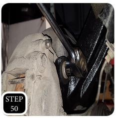
**STEP 50:** Unbolt the brake line bracket from the frame to gain some slack and attach the brake caliper to the steering knuckle.
