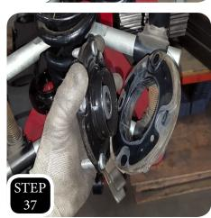
**STEP 37:** Remove the strut top and separate the rubber isolator from the top.
