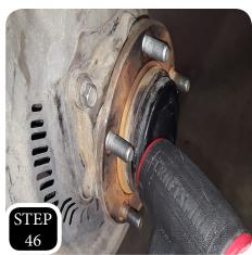
**STEP 46:** Install the castle retainer and the cotter pin and then re-install the dust cap onto the wheel bearing.
