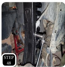
**STEP 47:** Attach the ABS sensor to the steering knuckle and tighten using the factory bolt.
