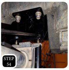
**STEP 54:** Attach the sway bar to the drop-down brackets using the provided 7/16" bolts, nuts, and washers, and tighten.
