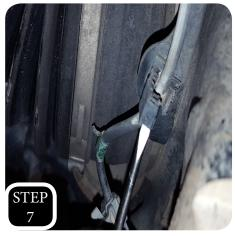
**STEP 7:** Separate the ABS line from both clips on the bracket at the front of the spindle.
