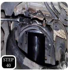
**STEP 40:** Attach the strut spacer to the top of the strut using the factory nuts and with the tall side facing outward. Next loosely attach the strut to the truck using the provided M10 flange nuts.
