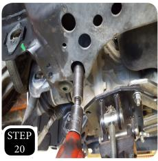
**STEP 20:**Unbolt both mounting bolts for the drive side rear diff mount and remove.
