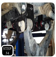
**STEP 34:** Loosely install the lower control arms into the subframe pockets using the factory alignment cams.
