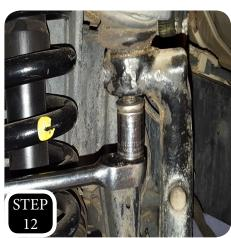
**STEP 12:** Remove the upper ball joint clip and loosen the nut, but do not remove.
