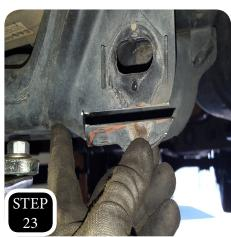
**STEP 22:** Cut across the line you just drew with a suitable cutting device and remove the excess material.
