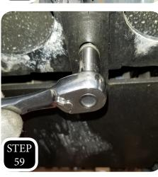
**STEP 59:** Install the skid plate using the provided 3/8" hardware up front and ½" hardware in the back and tighten.
