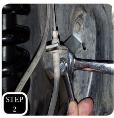
**STEP 52:** Attach the brake line extension bracket using the factory bolt at the frame and the provided M8-1.25 x 20 bolt, nut, and washer at the bracket.
