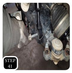
**STEP 41:** Swing the lower control arm up and loosely attach it to the strut using the factory hardware.
