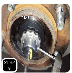
**STEP 9:** Remove the axle dust cap and then remove the cotter pin retaining the axle nut.
