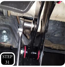
**STEP 31:** With all the diff mounts loosely attached, tighten the drive side rear diff mount to the diff.
