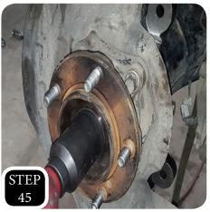
**STEP 45:** Install the wheel bearing with the factory dust shield and then tighten down the axle nut.
