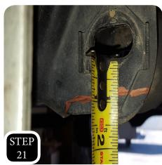
**STEP 21:** Measure ¾" down from the bolt hole of the front of the rear control arm pocket and mark a line parallel with slotted hole all the way across the flange.
