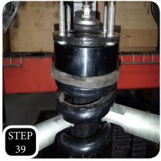
**STEP 38:** Install the Max Trac coil spacer in between the top and the isolator. **STEP 39:** Compress the coil a little further to make room for the coil spacer, then install the strut top with the coil spacer and tighten down the nut.
