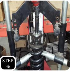
**STEP 36:** Compress the coil spring using a strut compressor and remove the upper retainer nut.
