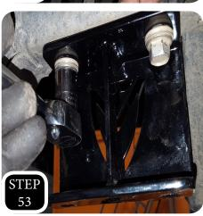
**STEP 53:** Remove the sway bar from the frame and attach the sway bar drop down brackets using the factory hardware with the Max Trac logo facing outward.
