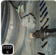
**STEP 8:** Unbolt the ABS sensor and support it up out of the way.
