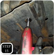
**STEP 15:** Unbolt all 5 skid plate bolts and remove the skid plate.
