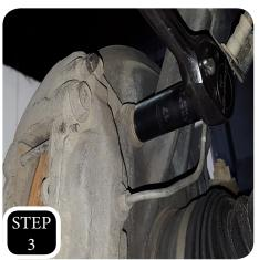
**STEP 3:** Unbolt both brake caliper bolts and support the caliper up out of the way.
