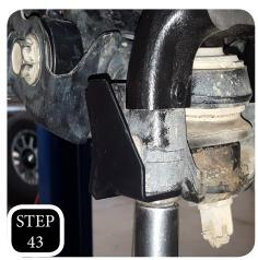
STEP 43: Attach the Max Trac steering knuckle to the truck and tighten. Make sure to attach the steering stop extension to the front lower knuckle bolt.
