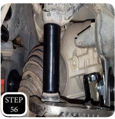
**STEP 56:** Remove the factory bump stops and install the tubular bump stop extensions, then tighten.
