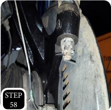
**STEP 58:** Once the tie rod ends have been swapped, tighten them down using the factory nuts and then install the cotter pin.
