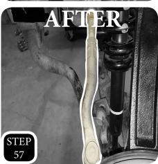
**STEP 57:** You will need to break the tie rod jam nut loose, unthread the tie rod, and swap the passenger side with the driver side.
