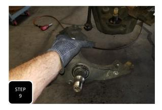
**Step 9** Lift up on the upper control arm and then remove the spindle.
