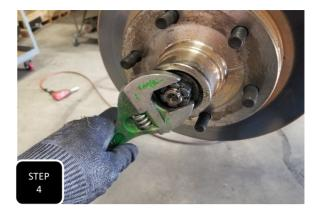
**Step 4** Remove the wheel bearing dust cap to access the wheel bearings. Next, remove the cotter pin from the castle nut and then loosen the castle nut.
