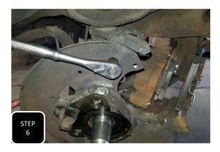
**Step 6** Remove the lower of the two ABS ring bolts along with the two dust shield bolts and remove them both.
