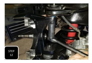
**Step 12** Torque the lower ball joint to 130 ft/lbs and the upper ball joint to 85 ft/lbs. Next, rotate the nut additionally until the hole in the ball joint aligns with the castle nut opening and then install the supplied cotter pin.
