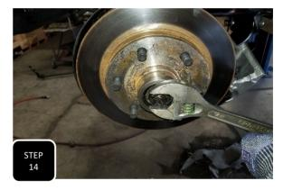
**Step 14** Install the rotor, bearings, washer and nut. Tighten down the nut to about 50 ft/lbs while spinning the rotor. This will seat the bearings.
