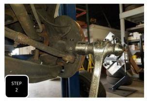
**Step 2** Pull the cotter pin from the castle nut at the tie rod, remove the nut, and then brake the rod end loose by hitting the side of the steering arm with a hammer. **NOTE: NEVER HIT THE ROD END ON THE THREADS.**
