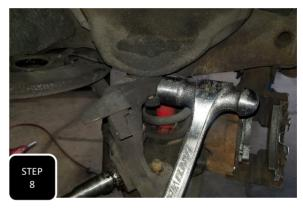
**Step 8** Remove the cotter pins for both the upper and lower ball joint nuts and then remove both ball joint nuts. Next, hit the side of the spindle, right at each ball joint, with a hammer to break the ball joint loose.
