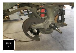
**Step 7** Remove the dust shield along with the ABS ring and support them out of the way.
