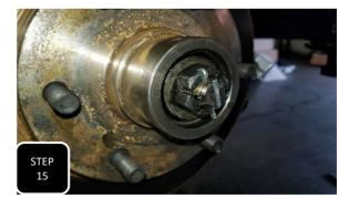
**Step 15** Loosen the nut and then tighten just beyond hand tight. Spin the nut a little bit tighter until the opening in the castle nut aligns with the hole in the spindle's spud and then install the provided cotter pin.
