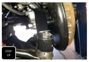
**Step 19** Install the tie rod from the bottom up and install the castle nut. Next, torque the nut to 50 ft/lbs then rotate the nut until the open slot of the castle nut lines up with the hole in the ball joint. Lastly, install the provided cotter pin. **REPEAT STEPS 1-19 ON THE OTHER SIDE.**
