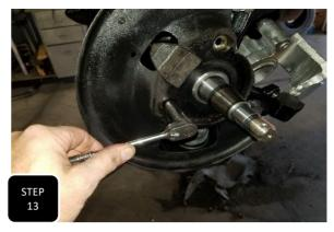
**Step 13** Install the dust shield along with the ABS ring using the factory bolts and tighten.
