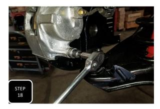
**Step 18** With the brake line now clear, tighten down both brake caliper mounting bolts.
