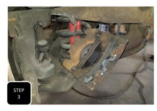
**Step 3** Unbolt both brake caliper mounting bolts and support the brake caliper up, out of the way. **NOTE: NEVER ALLOW THE BRAKE CALIPER TO HANG BY THE BRAKE LINE.**
