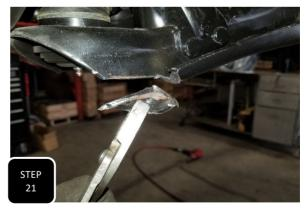
**Step 21** Mark about a 1.5" curved line across the end corner of the lower control arm lip and then using a suitable cutting device, remove this marked section. Next, clean up and round off all sharp edges and then spray paint for rust prevention.
