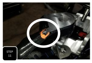
**Step 11** Check for contact with the upper control arm. If there is contact, mark the area and clearance using a suitable grinder and then re-install.
