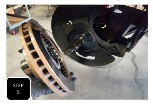
**Step 5** Remove the castle nut along with the outer wheel bearing and then remove the brake rotor.
