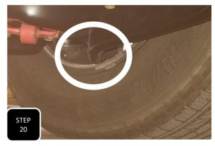
**Step 20** If you plan on running smaller than 20" rims then you will need to trim the lip of the lower control arm to prevent it from contacting the wheel at full turn.
