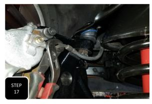
**Step 17** Loosely install the brake caliper over the rotor and you will see that the brake line hits the upper ball joint nut, preventing the caliper from sitting all the way down. Gently bend the hard brake line downward until the line clears the nut.
