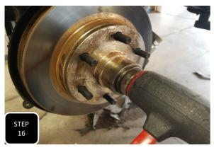
**Step 16** Re-install the dust cap over the wheel bearings using a mallet or dead blow to tap it into place.
