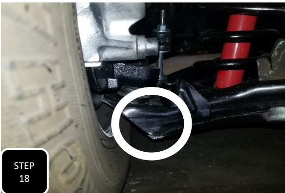
Step 18 If you plan on running smaller than 20" rims then you will need to trim the lip of the lower control arm to prevent it from contacting the wheel at full turn.
