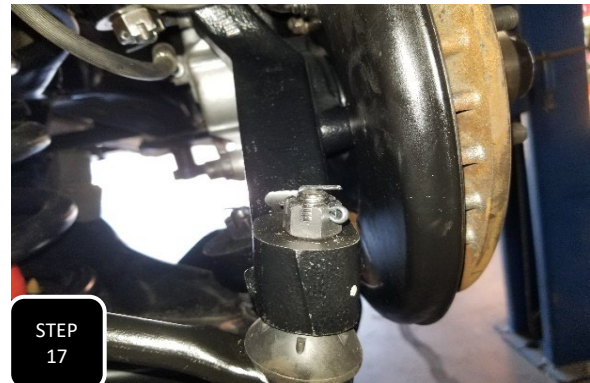
Step 17 Install the tie rod from the bottom up and install the castle nut. Next, torque the nut to 50 ft/lbs then rotate the nut until the open slot of the castle nut lines up with the hole in the ball joint. Lastly, install the provided cotter pin. REPEAT STEPS 1-17 ON THE OTHER SIDE.
