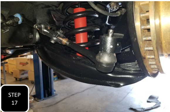
Step 17 Install the tie rod from the bottom up and install the castle nut. Next, torque the nut to 50 ft/lbs then rotate the nut until the open slot of the castle nut lines up with the hole in the ball joint. Lastly, install the provided cotter pin. REPEAT STEPS 1-17 ON THE OTHER SIDE.
