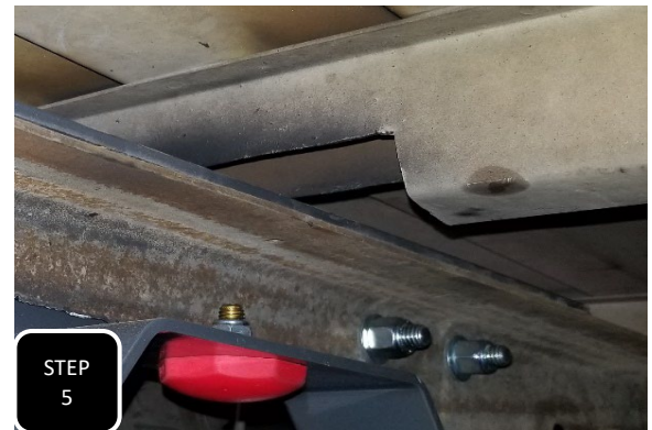
Step 5 Before being able to test fit the frame support, you will need to trim the bed rib, directly above, in order for the frame support to be able to slide over the top of the frame. Using a suitable cutting device, trim the bed rib about 1/2" up from the bottom. Trim from the end of the rib to at least the inside edge of the frame to ensure an easy install of the frame support and no contact of the two.
