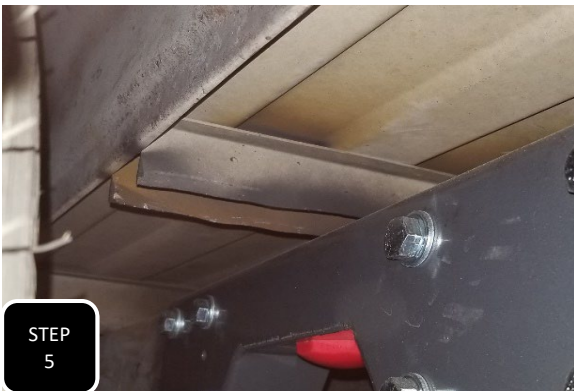
Step 5 Before being able to test fit the frame support, you will need to trim the bed rib, directly above, in order for the frame support to be able to slide over the top of the frame. Using a suitable cutting device, trim the bed rib about 1/2" up from the bottom. Trim from the end of the rib to at least the inside edge of the frame to ensure an easy install of the frame support and no contact of the two.
