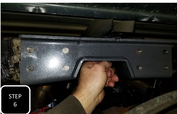
Step 6 Check for proper fitment and clearance as needed until the frame support fits flush to the frame. The longer, rectangular 4 bolt pattern goes towards the front of the truck and the square, 4 bolt pattern towards the rear.
