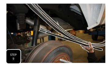
**Step 9** Unbolt the shackle mounting bolt and remove the front leaf spring bolt that you previously re-installed from the outside in, and then remove the leaf spring.
