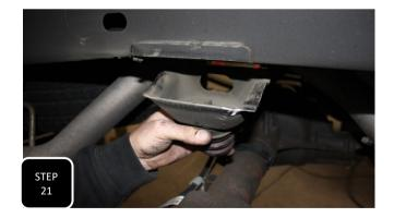
**Step 21** The factory bump stop extension bracket will need to be cut off the frame, so using a suitable cutting device, cut accross the outer mounting surface, inner mounting surface, and across the two bottom edges. Next, hit the bracket with a hammer and it should pop off. **NOTE: CONTROL THE DEPTH OF YOUR CUT SO THAT YOU DO NOT CUT THROUGH THE FRAME ITSELF.**
