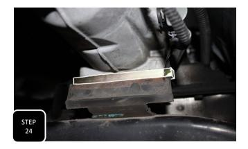
**Step 24** 2007-2013 models, install the gold, 1/2" tall transmission spacer between the trans and trans mount using the provided M10 bolts and washers. 2014-2018 models use the silver, 1/4" tall spacer. **NOTE: IF DRIVE LINE VIBRATION IS EXPERIENCED, YOU CAN ALTERNATE OR STACK SPACERS. IF VIBRATION PERSISTS, IT IS RECOMMENDED TO TAKE YOUR TRUCK TO A DRIVE LINE SPECIALIST.**
