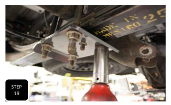
**Step 19** Place the provided U-bolt retainer plates on top of the factory spring perch with the bent ears facing in the direction of the front and back of the truck and then loosely install the factory U-bolts facing downward and through the provided spring plate under the leaf spring. Next, torque the U-bolts to 90 ft/lbs.
