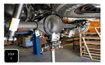
**Step 1** Jack up the rear of the vehicle and support under the frame rails with jack stands. Leave an adjustable jack under the differencial for height adjustment.
