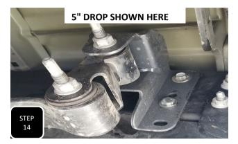
**Step 14** Attach the hanger with the shackle pre-assembled into it. The shackle will use the factory shackle bolt and can be installed with the open end facing either direction. The hanger will get attached using 3 of the provided 7/16" bolts and re-using the one factory bolt. **NOTE: THE SHACKLE CANNOT BE INSTALL AFTER THE HANGER IS INSTALLED.**
