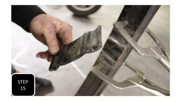
**Step 15** Install a couple clamps onto the leaf spring and remove the center pin. Next, remove and discard the U-bolt retainer plate and then re-install the center pin with the head on top of the leaf spring and the nut on the bottom. **NOTE: THIS IS OPPOSITE FROM THE WAY IT WAS ORIGINALLY INSTALLED.**
