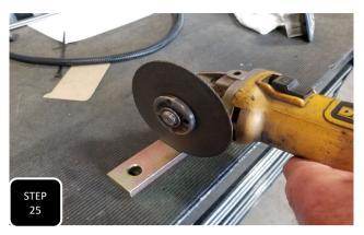
**Step 25** If drive line vibration is experienced on 4wd models, you will need to cut the provided spacer in half so that it will fit the bolt pattern of your T-case. It is recommended to start with the gold spacer. **NOTE: IF VIBRATION PERSISTS AFTER INSTALLING THE SPACER, IT IS RECOMMENDED TO TAKE YOUR TRUCK TO A DRIVE LINE SPECIALIST.**
