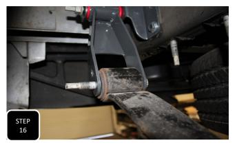
**Step 16** Jack the axle up and loosely attach the leaf spring to the shackle using the factory bolt facing from the inside, outward.
