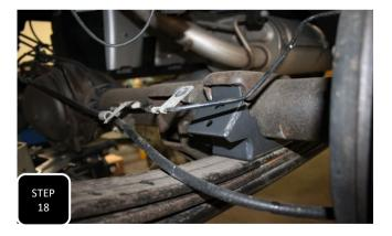
**Step 18** Once the axle is above the leaf spring on both sides and the leaf springs are both loosely installed, line up the provided axle relocators with the center pin on the spring and the attached brake line bracket facing the rear of the truck. Next, lower the axle into the relocators and assure the ears fit all the way up into the underside of the spring perch.
