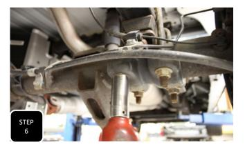
**Step 6** Remove the U-bolts and spring plates on one side only.
