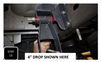
**Step 13** If installing the hangers in the 2 & 4 holes for a 4" or 6" drop, you will need to bend the bed seem, directly above the spring hanger, for additional clearance.
