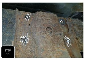
**Step 10** While the leaf spring is out, you will need to remove the rear, shackle hanger by making multiple cuts into the head of each of the 3 mounting rivots using a 4.5" cut off wheel. The bolt at the upper hole can just be un-bolted and saved for re-installation.
