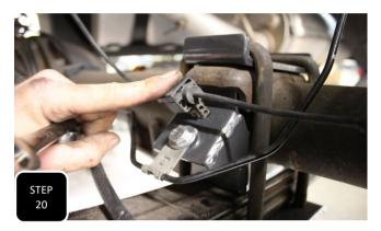
**Step 20** Attach the brake line guide bracket to the axle relocator using the provided M8 bolt, washer, and nut. Next, attach the ABS guide clip by pressing it into the slotted hole.
