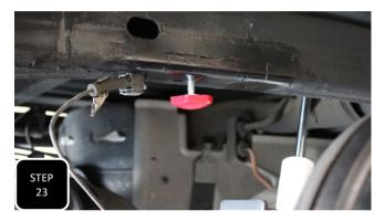
**Step 23** You also have the option of using the provided, low profile bump stop. If you choose to use this, then you will need to drill a 5/16" hole on your center mark and then tap that hole with a 3/8-16 tap. Next, thread the provided bump stop all the way up and hand tighten.
