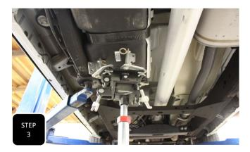
**Step 3** Since the front leaf spring bolts install from the inside of the frame, the gas tank will need to be removed to get this bolt out. Unbolt and remove the plastic skid plate then support the gas tank with a jack. **NOTE: THIS STEP IS EASIER WHEN GAS TANK IS CLOSE TO EMPTY.**
