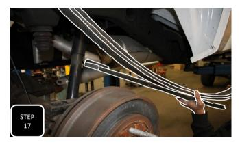
Step 17 Repeat steps 6-16 on the other side. NOTE: BE CAUTIOUS NOT TO STRETCH ANY ABS LINES OR BRAKE LINES AND IF PIVOTING THE AXLE SIDE TO SIDE, MAKE SURE IT IS SECURELY ATTACHED TO THE JACK.
