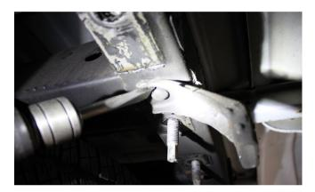
**Step 11** Next, you will need to chissel off the heads using a pneumatic hammer with a chissel attachment and then finally punch out the body of the rivot using a pneumatic hammer with a punch attachment. Older models will have one more rivot attaching a support bracket to the bottom of the frame. This bracket will be welded on newer models and needs to be cut off.
