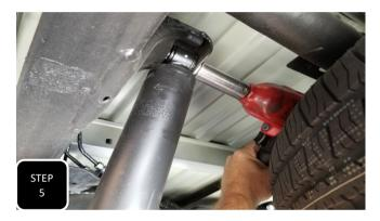
**Step 5** Once the gas tank is secure, move the jack back to the axle and jack it up slightly to apply pressure to the axle then unbolt both shocks at both ends and remove.
