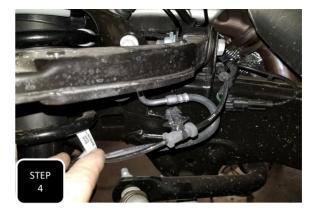
**Step 4** Separate the ABS wire mounting clip from the bracket on the upper control arm.
