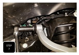
**Step 7** Locate the new upper control arm which has the ball joint off-set the same way as the arm you just took off. Now, loosely install the new arm using the factory bolts at the frame. **NOTE: DO NOT FULLY TIGHTEN THE BOLTS AT THE FRAME UNTIL THERE IS WEIGHT ON THE SUSPENSION LIKE THE TRUCK IS AT ITS NORMAL RIDE HEIGHT.**
