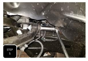
**Step 5** Loosen and remove both bolts attaching the upper control arm to the frame and save for re-installation.
