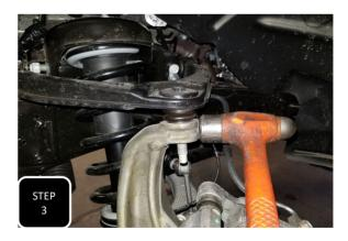
**Step 3** Unbolt the upper ball joint and break loose by hitting the side of the spindle, right at the ball joint, with a hammer, then separate.
