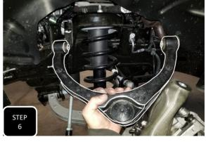
**Step 6** Pull the upper ball joint out of the spindle and gently allow the spindle to flop to the side. Next, remove the upper control arm.
