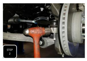
**Step 2** Unbolt the tie rod at the spindle and break loose by hitting the side of the spindle, right at the tie rod, with a hammer, then separate. **NOTE: NEVER HIT THE TIE ROD ON THE THREADS.**
