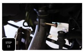
**Step 13** If replacing your upper control arms during this install, it is recommended to use **Motorcraft** brand arms as some after market control arms have been found to have a slightly smaller ball joint shank which could prove to not fully tighten up in your Max Trac lift spindle.
