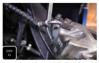
**Step 21** Loosely install the brake caliper onto the brake rotor. Using a pry bar, gently pry on the hard brake line, at the brake caliper, until the soft line clears the neck of the spindle.
