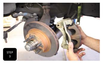
**Step 3** Unbolt both brake caliper mounting bolts and support the brake caliper up, out of the way. **NOTE: NEVER ALLOW THE BRAKE CALIPER TO HANG BY THE BRAKE LINE.**
