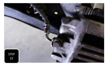
Step 22 Attach the caliper to the spindle using the factory bolts and tighten. NOTE: CHECK FOR PROPER BRAKE PAD ENGAGEMENT. IF THE BRAKE PADS ARE HANGING OFF THE END OF THE ROTOR BY ABOUT 1/2" THEN YOU HAVE THE WRONG SPINDLES. 1998-2000 MODELS HAD A 10.280" DIAMETER ROTOR WHERE AS 2001-2009 MODELS HAD A 11.280" ROTOR.
