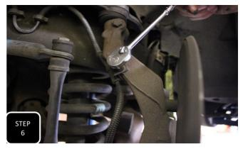
**Step 6** Unbolt the ABS sensor from the spindle and then unbolt the ABS wire guide from the neck of the spindle. Next, hang the ABS sensor up, out of the way so that it does not get damaged during the install.
