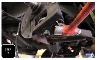
**Step 7** Remove the cotter pin from the lower ball joint, loosen but don't remove the nut and then break the ball joint loose by hitting the side of the spindle, right at the ball joint. **NOTE: NEVER HIT THE BALL JOINT ON THE THREADS.**
