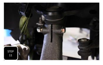
**Step 11** Loosely install the new spindle by tightening the LBJ nut and just loosely installing the UBJ bolt. Cycle the spindle back and forth in its steering cycle to make sure the control arm has been clearance enough. If there is still contact, remove the spindle and clearance a little more. **NOTE: TORSION BAR RANGER'S HAVE A LARGER UPPER BALL JOINT THAT WILL NOT FIT IN THE HOLE OF A COIL SPRING RANGER SPINDLE. SEE MEASUREMENTS ARE ON THE COVER PAGE OF THESE INSTRUCTIONS.**
