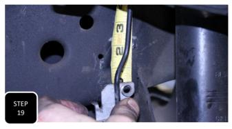
**Step 19** Locate where the soft brake line meets the hard brake line and unbolt the mounting bracket from the frame. Mark a spot 2 1/8" straight down from the original bolt hole.
