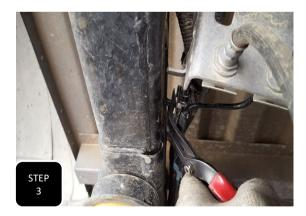
Step 3 Unbolt the brake line bracket from the frame and the support clip just behind it.
