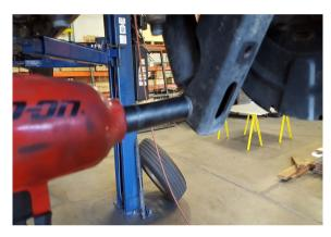
**Step 2** Apply pressure to the bottom of the axle then unbolt both shocks from the axle and save hardware for reinstallation. If you have new shocks to install, unbolt both shocks from both ends and remove.
