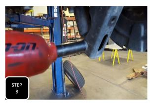
**Step 8** Re-attach the shocks to the axle or if installing new shocks, do so at this time and tighten.
