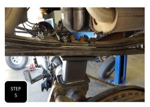
**Step 5** Install the new block with short side facing forward and bump stop striker plate facing inward. **NOTE: THESE BLOCKS HAVE ANGLE BUILT INTO THEM AND MUST BE INSTALLED WITH THE SHORT SIDE FACING FORWARD AND THE TALL SIDE FACING REARWARD.**
