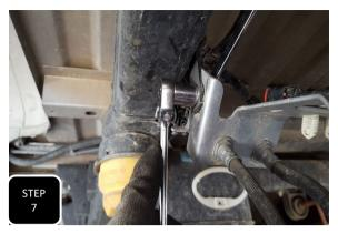
**Step 7** Gently bend the brake lines downward and loosely install the brake line drop down bracket using the factory bolt at the frame and the provided bolt at the bracket. Once aligned, tighten down both bolts.
