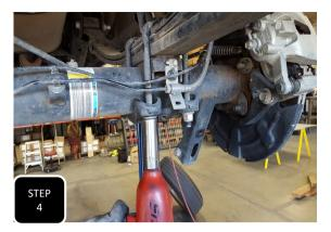
**Step 4** One side at a time, remove the U-bolts and lower the axle to make room for the lift block. **NOTE: MAKE SURE THAT NONE OF THE BRAKE LINES OR ABS LINES GET STRETCHED WHEN LOWERING THE AXLE.**
