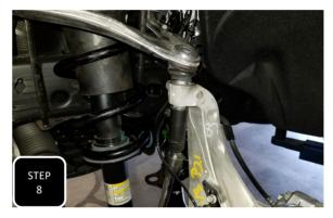
**Step 8** Loosely install the top of the strut in the truck using the provided flange nuts. Next, place a floor jack under the lower control arm, remove the upper control arm nut, and then allow the lower control arm to go down until the bottom of the strut aligns above the control arm. **NOTE: MAKE SURE TO KEEP THE TOP OF THE SPINDLE FROM FLOPPING SO THAT THE BRAKE LINE OR ABS LINE DO NOT GET TORN OR STRETCHED.**
