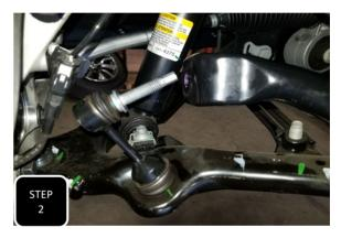
**Step 2** Remove the nut attaching the sway bar end link to the sway bar and separate the two.
