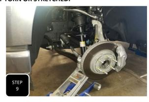
**Step 9** Install the lower strut bolts and tighten. Next, apply pressure to the control arm with the jack and compress the coil until you are able to re-attach the spindle to the upper control arm. Torque to factory specs.
