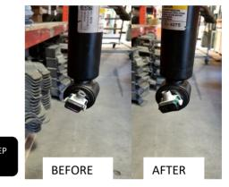
**Step 5** Using an automotive coil/strut compressor, compress the coil so that the bottom of the strut can be rotated 180 degrees. **NOTE: THE LOWER BAR PIN IS VULCANIZED AT AN ANGLE AND NEEDS TO BE ROTATED TO ANGLE IT IN THE PROPER DIRECTION AFTER INSTALLING THE STRUT SPACER.**
