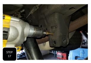
**Step 17** Using a scribe, trace the upper, side hole of the trac bar bracket, then remove the bracket and drill a 1/2" hole through your circle.
