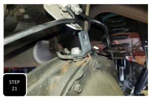
**Step 21** Remove the "O" ring that is on the factory mounting bolt for the brake line bracket at the top of the diff. Next, attach the provided brake line bracket to the top of the diff using this bolt and tighten.
