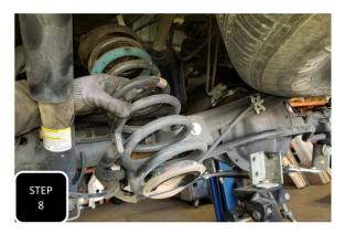
**Step 8** Lower down the axle and remove both coil springs. **NOTE: MAKE SURE TO SAVE THE RUBBER ISOLATORS FOR RE-INSTALLATION.**
