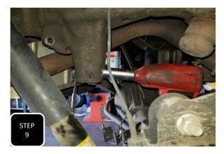
**Step 9** Unbolt the trac bar from the mount on the frame and separate.
