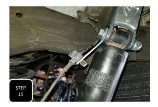
**Step 15** Loosely install the provided shock extenders with the logo facing outward, using the factory shock bolt. Next, attach the shock to the extender using the provided 14mm bolt, nut and washer and fully tighten both bolts. **NOTE: ON THE DRIVER'S SIDE, YOU WILL ATTACH THE PROVIDED ABS LINE BRACKET TO THE SHOCK MOUNTING BOLT AT**
