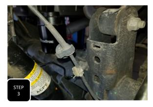
**Step 3** Unclip the ABS line guide clips from the back side of the upper control arm mounts on both sides.
