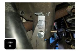
**Step 18** Re-install the bracket using the provided zinc plated crush tube and 14mm hardware. Next, install the provided 7/16" bolts, nuts, and washers through the two side holes. You will also be attaching the provided pass side ABS line bracket to the upper bolt with the "D" shaped hole facing upward, then tighten all 3 bolts.
