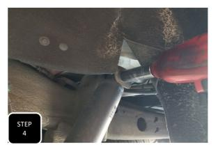
**Step 4** First, apply pressure to the diff with the adjustable jack. Next, to access the upper shock mount more easily, cut a slit in the wheel well liner and remove the upper mounting bolt of the shock.
