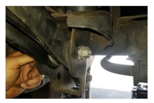
**Step 14** Loosely re-attach the lower control arm to the axle and only snug up the nuts. **NOTE: THESE BOLTS WILL GET FULLY TIGHTENED WHEN THE TRUCK IS BACK ON THE GROUND AT RIDE HEIGHT.**
