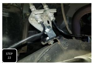
**Step 22** Gently bend the hard brakelines until the factory mounting bracket is vertical and the soft brakelines are pointed straight up. Next, attach the factory brakeline bracket to the provided brakeline bracket using the provided 8mm bolt, nut, and washers.
