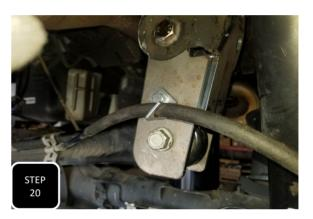
**Step 20** Slide the E-brake guide bracket onto the E-brake cable near the trac bar bracket on the passenger side and then attach this bracket to the small hole on the back of the trac bar bracket using the provided 8mm bolt nut and washers. **NOTE: DO NOT FULLY TIGHTEN THIS BRACKET. ONLY SNUG IT UP AS IT WILL NEED TO PIVOT AS THE SUSPENSION CYCLES.**
