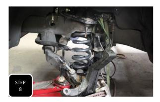
**Step 8** Get the spring into place and apply some tension with the floor jack. Next, use a large pry bar to apply inward pressure on the spring while you jack the lower control arm up. Once the control arm is flat, the coil spring will no longer want to pop out and the pry bar can be removed. **NOTE: THE USE OF AN INTERNAL COIL COMPRESSOR, OTC PART # 7045B WILL GREATLY EASE THE INSTALL PROCESS.**
