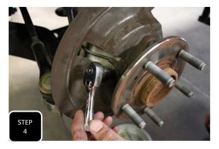
**Step 4** Unbolt the ABS sensor from the spindle or hub and swing it out of the way so that it does not get damaged during the install.
