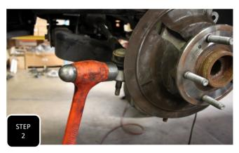
**Step 2** Unbolt the tie rod and break it loose by hitting the side of the spindle, right at the tie rod, with a hammer. **NOTE: NEVER HIT THE TIE ROD ON THE THREADS.**
