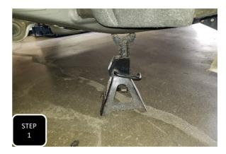
**Step 1** Jack up the front of the truck and support under the frame rails with jack stands. Keep the floor jack under the lower control arm for height adjustment during the install.
