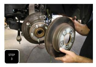
**Step 3** Unbolt the brake caliper and support out of the way. Next, remove the brake rotor. **NOTE: NEVER ALLOW THE BRAKE CALIPER TO HANG BY THE BRAKE LINE.**
