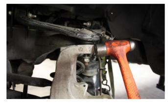
**Step 6** Place a floor jack under the lower control arm and apply some pressure. Next, remove the upper ball joint nut and break the ball joint loose by hitting the side of the spindle, right at the ball joint, with a hammer. **NOTE: NEVER HIT THE BALL JOINT ON THE THREADS.**
