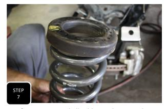
**Step 7** Lower the jack down and remove the stock coil spring. Transfer over any and all rubber isolators to the new coil spring and install the spring. **NOTE: FACTORY ISOLATORS ARE ALWAYS RUBBER AND ARE USUALLY ABOUT 1/4" THICK ABOVE THE SPRING. ANYTHING THICKER IS A LIFT SPACER AND NEEDS TO BE DISCARDED.**
