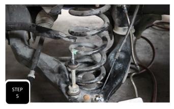
**Step 5** Unbolt the sway bar from the sway bar end link.
