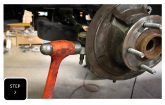
**Step 2** Unbolt the tie rod and break it loose by hitting the side of the spindle, right at the tie rod, with a hammer.
