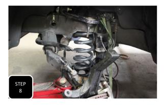
**Step 8** Get the spring and spacer into place and apply some tension with the floor jack. Next, use a large pry bar to apply inward pressure on the spring while you jack the lower control arm up. Once the control arm is flat, the coil spring will no longer want to pop out and the pry bar can be removed. **NOTE: THE USE OF AN INTERNAL COIL COMPRESSOR, OTC PART # 7045B WILL GREATLY EASE THE INSTALL PROCESS.**
