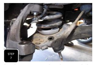
**Step 7** Lower the jack down and remove the stock coil spring. Place the new spacer on the coil groove in the lower control arm and then place the spring on top of it. **NOTE: THE SPRING WILL NOT BE FLAT ON THE SPACER RIGHT NOW BECAUSE THE CONTROL IS AT A STEEP ANGLE FROM BEING DROOPED OUT.**
