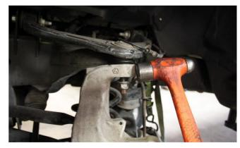
**Step 6** Place a floor jack under the lower control arm and apply some pressure. Next, remove the upper ball joint nut and break the ball joint loose by hitting the side of the spindle, right at the ball joint, with a hammer.
