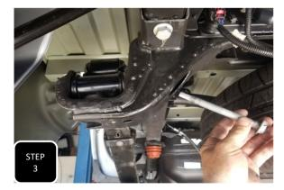
**Step 3** First remove the lower shackle bolt on both sides and then jack the axle up until the eye of the leaf spring hits the bottom of the bed.
