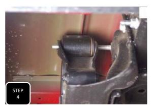
Step 4 Remove the upper bolts and then the shackles. NOTE: If there is a bed seam directly above the shackle, then it will need to be cut and bent in order to get the bolt high enough to remove between the bed and top of the frame. F-150's will require the bed bolts to be loosened and the bed to be lifted up.
