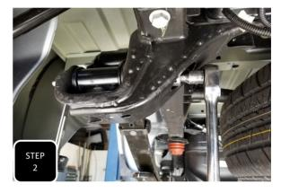
Step 2 Remove the nuts from both shackle bolts on both sides and set aside for re-installation.
