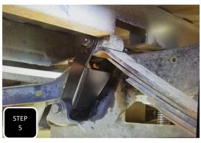
Step 5 Certain applications will require a bed rib to be cut and removed if it is above the shackle and the shackle is long enough to contact it. Cut a suitable section out and then install the new shackle. NOTE: SOME APPLICATIONS, SUCH AS F-150'S, HAVE THIS BED RIB ABOVE THE SHACKLE WHICH WILL PREVENT THE SHACKLE FROM GOING HIGH ENOUGH TO REMOVE THE BOLT. THE BED WILL NEED TO BE LOOSENED AND LIFTED IN ORDER TO REMOVE THE SHACKLE TO SPRING BOLT.
