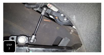
**Step 2** Remove the factory sensor rods attached towards the front of upper link arms by using a prefered prying tool to pop the plastic rod end off of the attached metal ball.
