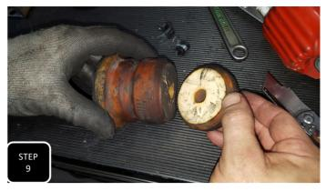
**Step 9** If installing a 3" or 4" drop, you will need to pop the factory bump stop out of its mount on the frame and cut off one rib so that the bump stop does not prevent the truck from achieving its full amount of drop.
