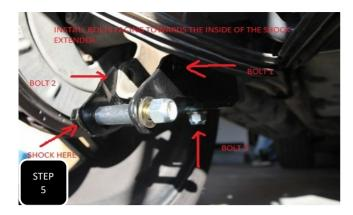
**Step 5** Install the provided shock extenders over the factory shock mounts on the axle. Use the provided 1/2" bolts through the original shock mount holes, from the outside facing in along with the provided lock washers and jam nuts. Next, us the longer 1/2" bolt to attach the back of the extender up through the bottom of the factory mount and tighten the bottom bolt first and then the side bolts.
