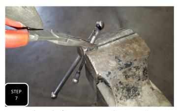
NOTE: THE FACTORY ROD ATTACHES TO THE PLASTIC ROD END VIA A RETAINER LIP AND GROOVE IN THE ROD. THE MAXTRAC REAR SENSOR RODS ARE THREADED FOR ADJUSTABILITY OF RIDE HEIGHT.
