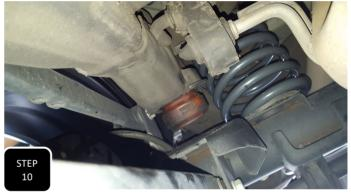
Step 10 Once cut, re-install the bump stops and there should be about 1-2" of gap depending on the amount of drop.
