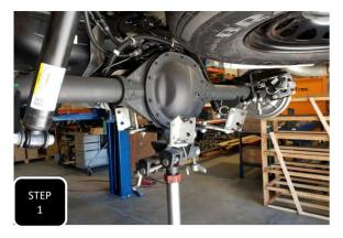
**Step 1** Jack up the rear of the vehicle and support under the frame rails with jack stands. Leave an adjustable jack under the diff for height adjustment.
