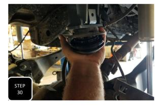
**Step 30** Attach the factory bump stop mounting cup to the bottom of the drop down bracket using the provided M8 bolt, nut, and washers. Once tight, then pop the factory bump stop back in. On the driver's side, you will attach the provided Vacuum line mounting bracket as pictured. **NOTE: SPRAY THE BUMPS STOP WITH WD-40 TO EASE THE INSTALL PROCESS.**
