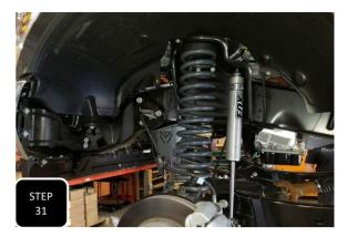
**Step 31** Move your adjustable jack under the driver's side of the axle and apply pressure so that you can remove the lower shock bolt and then lower the axle down. Next, Install the new lift coil with the factory rubber isolator on top, jack the axle back up and re-attach the shock. Repeat this step on the other side.
