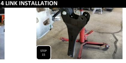
**Step 15** Loosen all 3 radius arm mounting bolts, 2 at the axle and 1 at the frame and then remove the radius arm. **NOTE: WORK ON ONE SIDE AT A TIME.**
