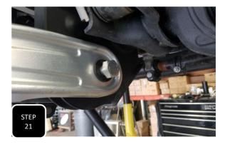
**Step 21** Remove the upper bolt attaching the radius arm on the other side so that the axle can be rotated. Next, insert two of the larger sleeves into the hole in the lower link and attach the lower link to the axle using the provided M18 bolt, nut, and washers. **NOTE: DO NOT FULLY TIGHTEN THESE BOLTS UNTIL THE TRUCK IS BACK ON THE GROUND AT RIDE HEIGHT.**
