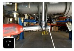
Step 8 Install your new longer shocks using the factory hardware and tighten. NOTE: MAX TRAC SHOCKS HAVE TO BE MOUNTED WITH THE BODY OF THE SHOCK AT THE AXLE AND THE SHAFT OF THE SHOCK AT THE FRAME. FOX SHOCKS WILL BE MOUNTED THE OPPOSITE OF THIS.
