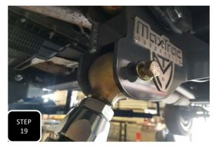
**Step 19** Locate the other arm that matches the one you just installed, adjust it to an eye-eye length of 32" and grease the rod end. Next, loosely install it into the bottom hole of the 4 link frame bracket using the provided 9/16" bolt, washers, and nut. **NOTE: THE ROD ENDS ARE NOT PRE-GREASED AND REQUIRE GREASE FOR PROPER FUNCTION.**
