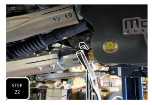
**Step 22** Tighten down all 4 of the M8 pinch bolts and then cinch down the two jam nuts on the rod ends. Repeat steps 15-22 on the other side.
