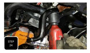
**Step 24** Apply a conservative amount of thread locker to the threads of the factory nut then attach the new drop down pitman arm to the steering box using the factory nut. Once tight, then torque to 350 ft/lbs. **NOTE: MAKE SURE TO INSTALL THE NEW PITMAN ARM IN THE EXACT SAME DIRECTION AS THE OLD ONE CAME OFF.**
