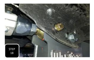
**Step 18** Locate 1 of the 4 arms. There should be 2 DS where the "MT" logo is facing up and the pinch bolts are facing outward. The PS arms are the opposite. Adjust the arm to a length of 32" from eye-eye with the grease fitting facing downward. Next, grease the rod end and loosely install it into the upper part of the 4 link frame bracket where you previously loosely installed the provided 9/16" bolt. **NOTE: THE ROD ENDS ARE NOT PRE-GREASED AND REQUIRE GREASE FOR PROPER FUNCTION.**
