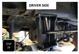
**Step 29** Pop the factory bump stop out of its mounting cup then unbolt the cup and using the same bolt, attach the new bump stop drop down bracket to the same mounting hole. The angled side of the bracket will face the rear of the truck, the shorter of the two surfaces downward, and the open end outward.
