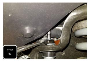
**Step 32** Tighten up both ends of both front shocks.
