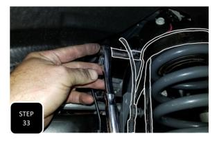
**Step 33** Separate both ABS line guide clips from the front of the coil bucket on the frame and install the new ABS/brake line bracket using the provided M8 bolts, nuts, and washers. **NOTE: THE DRIVER'S SIDE BRACKET IS THE LONGER OF THE TWO PROVIDED BRACKETS.**
