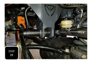
**Step 39** When attaching the trac bar to the drop down bracket, you will need to use the provided off-set plates. The hole will need to be off-set to the driver's side for the 4" lift or towards the passenger side for the 8" lift. Use the factory M18 bolt and nut and only loosely attach for now. **NOTE: THE TRAC BAR WILL GET FULLY TIGHTENED WHEN THE TRUCK IS ON THE GROUND AT RIDE HEIGHT.**
