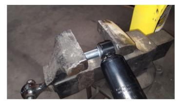
**Step 7** If installing Max Trac shocks, you will need to grease the bushings and use a bench vise to press in the shock sleeves.
