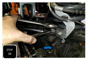
**Step 38** Attach the sway bar to the drop down brackets using the provided M10 bolts, nuts, and washers then tighten. Next, re-attach the ends to the end links on the axle using the factory nuts and tighten.
