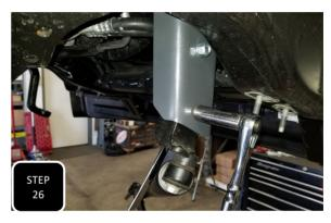
**Step 26** Using the provided M10 bolts and washers, attach the new steering stabilizer drop down bracket to the inside of the passenger side frame with the welded shim touching the frame and tighten. Next, attach the factory bracket to the lower half of the drop down bracket using the other provided M10 bolts, nuts, and washers. **NOTE: THE FACTORY BRACKET WILL MOUNT INSIDE OF THE PROVIDED BRACKET.**
