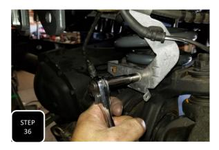
**Step 36** Using the factory bolt, re-attach the brake line bracket to the lower coil mount as it was originally.
