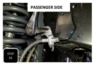
**Step 35** The passenger side ABS/ brake line bracket will mount the same as the driver's side and also require the unraveling of the factory hard brake line to line up with the new bracket.
