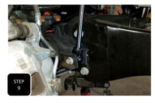
**Step 9** Loosely attach the new shock to hold the axle, then move the jack to the passenger side and repeat steps 6-9. **NOTE: THE SHOCKS WILL HOLD THE AXLE AS YOU MOVE THE JACK AND CONTINUE THROUGH THE INSTALL.**
