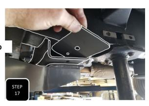
**Step 17** Locate the flat plate labeled DS and slide it into the cross member above the back of the 4 link bracket. Line up the holes and loosely attach the plate and bracket together using the provided 3/8" and 5/16" socket head allen bolts. **NOTE: THE DRIVER'S SIDE IS THE LONGER PLATE**
