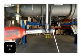
Step 9 Install your new longer shocks using the factory hardware and tighten. NOTE: MAX TRAC SHOCKS HAVE TO BE MOUNTED WITH THE BODY OF THE SHOCK AT THE AXLE AND THE SHAFT OF THE SHOCK AT THE FRAME. FOX SHOCKS WILL BE MOUNTED THE OPPOSITE OF THIS.
