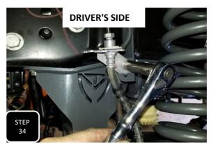
**Step 34** You will need to gently unravel the factory, hard brake line so that the soft line now points downward and the factory mounting bracket lines up with the two holed flange on the provided mounting bracket. Next, attach the factory bracket to the provided bracket using the provided M8 bolt, nut, and washers.
