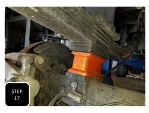
**Step 17** Install the new lift block. The block is flat so it can be installed either way. Align the center pins and jack up the axle to seat the block.
