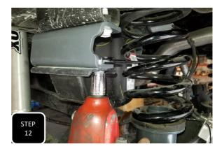
**Step 12** Unbolt the factory bump stops and install the bump stop extension brackets with the notched edge facing the back of the truck and the open end facing inward. Next, attach the factory bump stops to the new bracket using the provided M10 hardware and tighten.
