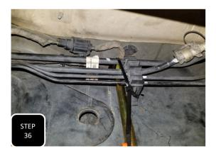
**Step 36** Use the supplied zip tie to attach the fuel line assembly to the U-bolt.
