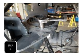
Step 8 Tighten up the two 3/8" bolts. NOTE: THE EASIEST WAY TO TIGHTEN DOWN THE BOTTOM 3/8" BOLT IS TO STICK A FLAT HEAD SCREW DRIVER DOWN INSIDE THE BRACKET AND WEDGE IT AGAINST THE HEAD OF THE BOLT WHILE TIGHTENING THE NUT WITH A RATCHET.
