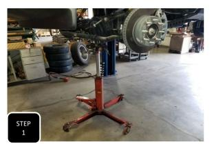
**Step 1** Jack up the front end of the vehicle and support under the frame rails with jack stands. Keep an adjustable jack under the axle for height adjustment.
