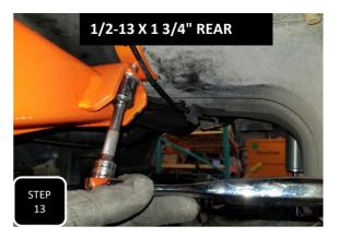
**Step 13** Slide the trac bar attachment plate between the oil pan and the cross member and loosely attach with the provided  $1/2-13 \times 1 \ 1/2$ " bolt at the front and  $1/2-13 \times 1 \ 3/4$ " bolt at the rear. Next, tighten down all 4 mounting bolts. **NOTE: THE ANGLED SIDE OF THE ATTACHMENT PLATE POINTS FORWARD.**
