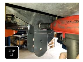
**Step 19** Loosely install the new radius arm bracket into the factory mount using the factory radius arm bolt in the main hole and the supplied hardware for the U-bolt. Push the bracket up tight against the frame and tighten the U-bolt first, then tighten the stock mounting bolt. Once tight, torque the factory bolt to factory specs and the U-bolt to 100 ft/lbs.
