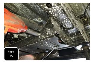
**Step 25** Remove the mounting nuts for the cross member just inside the radius arm bracket and push the bolts back so that the heads are not sticking out of the cross member.
