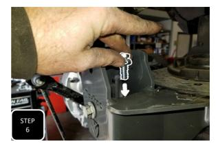
**Step 6** Slide the new trac bar bracket over the factory trac bar bracket on the axle and loosely install the factory bolt through the original trac bar mounting hole with the provided crush tube in the middle. Next, install one of the provided 3/8" bolts and washers through the inside, bottom of the bracket.
