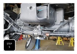
**Step 5** Dis-engage the guide clip attaching the brake line to the bottom of the trac bar bracket and pull down a bit so it is out of the way.
