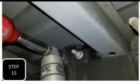
**Step 15** Jack up the rear of the truck and support under the frame with jack stands. Apply pressure to the rear diff with an adjustable jack and remove both rear shocks.
