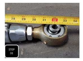
**Step 31** Adjust the upper links to 28.5" (the shorter link) and the lower links to 32" (the longer link). Now locate the links for the side that you are working on first. The driver's side links, when installed will have the Max Trac logo facing upright and the two pinch bolts facing outward when installed. **NOTE: THE LENGTH OF THE ARMS IS MEASURED FROM CENTER OF MOUNTING HOLE.**
