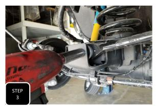
**Step 3** Unbolt the trac bar from the bracket on the axle and separate.
