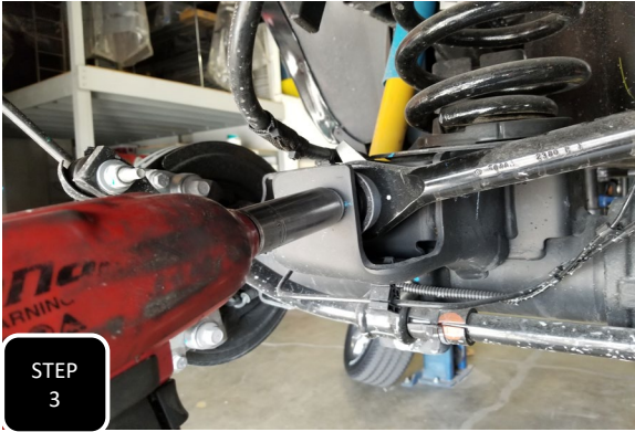
Step 3 Unbolt the trac bar from the bracket on the axle and separate.
