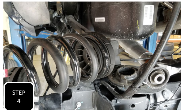
Step 4 Unbolt the sway bar end links from the frame on both sides and spin them out of the way. Next, lower the axle and remove both of the rear coils.
