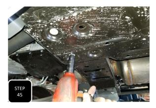
**Step 45** Re-attach the brake line brackets to the top of the axle and ensure that the brake lines are not tight when the suspension is at full droop. Next, re-install the skid plate under the transfer case and tighten.
