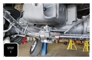
**Step 7** Disengage the guide clip attaching the brake line to the bottom of the trac bar bracket and pull down a bit so it is out of the way.
