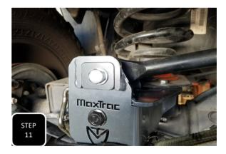
**Step 11** The plates with the off-center hole will get installed with the bolt towards the passenger's side for the 8" lift. Its only off-set to the drive side for the 4" & 6" lift. **NOTE: DO NOT TIGHTEN UNTIL THE TRUCK IS ON THE GROUND AT RIDE HEIGHT.**
