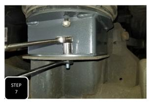
**Step 7** Tighten down the studs at the air bags using the factory nuts. Next, attach the spacers to the axle using the provided M8 bolts, nuts and washers then tighten.
