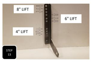
**Step 13** There are 9 mounting holes on the new sensor bracket. The 3 lowest holes are for a 1.5" rear lift, the 3 middle holes are for a 3.5" rear lift, and the 3 upper holes are for a 5.5" rear lift. Install the factory mounting ball into the desired hole using the provided M6 nut and washer then attach the sensor rod to it. **NOTE: THE MIDDLE HOLE OF EACH SET OF HOLES IS THE STARTING HOLE AND THE ABOVE OR BELOW HOLES WILL LIFT OR LOWER THE REAR OF THE**
