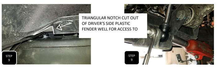
Step 9 Install the new shocks and tighten down both ends. NOTE: DO NOT OVER TIGHTEN THE TOP BUSHING OF THE SHOCK OR THE BUSHING WILL NOT BE ABLE TO FLEX AND COULD DAMAGE TO THE SHOCK.
