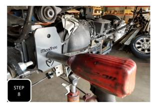
**Step 8** Tighten down the 3/8" bolt at the bottom of the trac bar bracket. The easiest way to hold the head of the bolt tight is to wedge a flat head screw driver down against the head. Next, tighten down the bolt in the original trac bar mounting hole.
