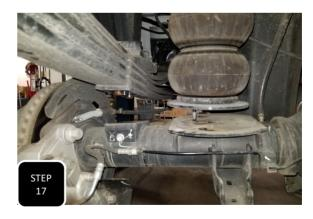
**Step 17** One side at a time, loosen both U-bolts, remove the U-bolts, and lower the axle to make room for the lift block. **NOTE: IT WILL HELP THE ALIGNMENT OF THE LIFT BLOCK TO SLIGHLY LOOSEN THE U-BOLTS ON THE OTHER SIDE.**
