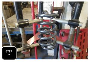
**Step 7** Remove the factory spring from the strut compressor, locate your new lowering spring, and compress it in the spring compressor.
