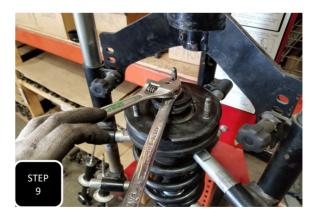
**Step 9** Re-install the strut top and tighten down using the factory nut. **NOTE: MAKE SURE TO PROPERLY CLOCK THE STRUT TOP WITH THE BOTTOM OF THE STRUT.**
