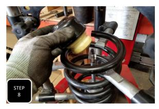
**Step 8** Slide the strut up into the coil and then slide the bump stop onto the shaft of the strut.
