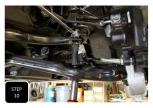
**Step 10** Reverse steps 2-9 and then repeat on the other side. **NOTE: DO NOT RE-ATTACH THE SWAY BAR END LINKS UNTIL BOTH SIDES HAVE BEEN INSTALLED.**
