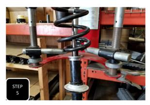
**Step 5** Once the nut is removed, pull the strut top off, remove the bump stop and remove the strut out the bottom of the coil. **NOTE: FOR SOME YEAR RANGES, THE BUMP STOP CUP IS ONE PIECE WITH THE STRUT TOP.**
