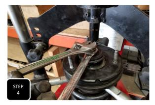
**Step 4** Using an automotive coil/strut compressor, compress the coil so that the strut can be disassembled safely and then remove the nut at the center of the strut top. **NOTE: PAY ATTENTION TO THE ORIENTATION OF THE STRUT TOP TO THE BOTTOM BARPIN FOR RE-ASSEMBLY.**
