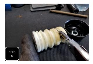
**Step 6** Locate the factory bump stop, remove it from the metal cup, and cut one rib off of the end of it.
