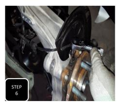
Step 6 Unbolt the ABS sensor from the spindle and swing it safely out of the way.
