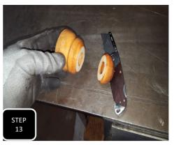
**Step 13** Cut down the factory bump stop by one rib and slide the bump stop onto the shock shaft.
