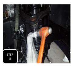
**Step 8** Loosen the upper ball joint then hit the side of the spindle with a hammer to break the ball joint loose. The nut will catch the spindle, then separate. **NOTE: NEVER HIT THE BALL JOINT ON THE THREADS.**
