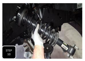
**Step 10** Remove both lower and all three upper strut mounting nuts and remove the strut. You will need to pry down on the lower control arm then pivot the strut out of the upper mount. Next lift up and remove.
