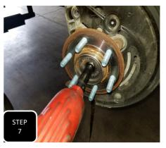
**Step 7** For 4wd models, remove the dust cap at the middle of the wheel bearing and then remove the axle retaining nut.
