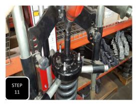
**Step 11** Using an automotive coil.strut compressor, compress the coil so that the strut can be disassembled safely and then remove the nut at the center of the strut top. **NOTE: TAKE NOTE OF THE POSITION OF THE STRUT TOP AND BOTTOM IN RELATIONSHIP TO EACH OTHER.**
