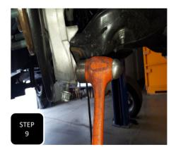
**Step 9** Loosen the lower ball joint then hit the side of the spindle with a hammer to break the ball joint loose. The nut will catch the spindle, then separate. **NOTE: NEVER HIT THE BALL JOINT ON THE THREADS.**
