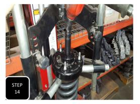
**Step 14** Re-install the strut into the coil and assemble then tighten down the top nut. **NOTE: MAKE SURE THE TOP, 3 BOLT PATTERN IS IN THE SAME RELATION TO THE BOTTOM AS IT WAS WHEN YOU TOOK IT APART.**
