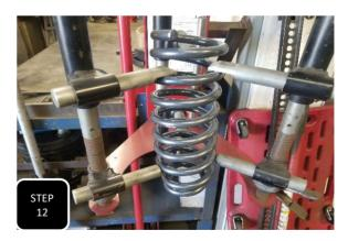
**Step 12** Remove the strut and set off to the side. Uncompress the coil spring, locate the new lowering spring, and install that in your spring compressor.
