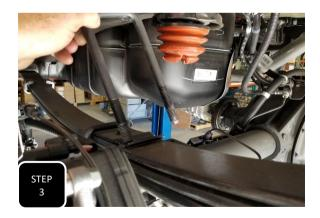
**Step 3** Unbolt the factory U-bolts, only on one side, and lower the axle enought to fit the new lift block between the axle and leaf spring. **NOTE: KEEP AN EYE ON ALL BRAKE LINES, ABS LINES, AND WIRES TO MAKE SURE THEY DO NOT GET STRETCHED OR DAMAGED.**
