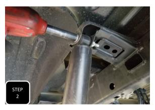
Step 2 Unbolt both shocks at both ends and remove. Save the factory hardware for the installation of the new shocks.
