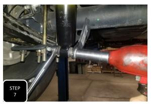
**Step 7** Install your new, longer shocks or factory shocks with a shock extender at this time using the factory bolts. **NOTE: IF THERE IS A GAP BETWEEN THE SHOCK BUSHING AND SHOCK MOUNTING EAR, IT WILL HELP TO INSTALL A WASHER NEXT TO THE BUSHING.**
