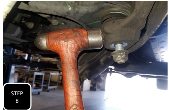
Step 8 Brake each ball joint loose by hitting the side of the spindle with a hammer, right at the ball joint. The nut will catch the spindle, then remove the spindle.
