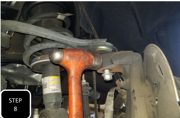
Step 8 Brake each ball joint loose by hitting the side of the spindle with a hammer, right at the ball joint. The nut will catch the spindle, then remove the spindle.
