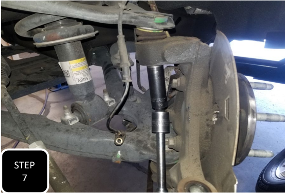
Step 7 Loosen both the upper and lower ball joint nuts, but do not remove.
