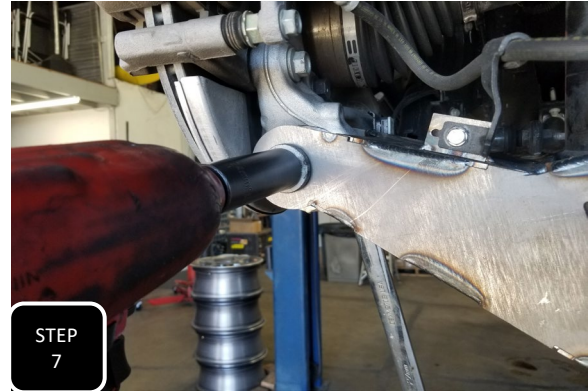
Step 7 Attach the control arm to the spindle using the factory bolt and provided M18 nut/washer then fully tighten to factory specs.
