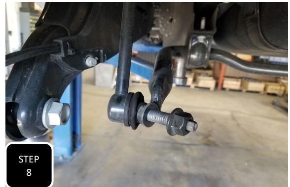
Step 8 Unbolt the sway bar end link from the sway bar on the side you are working on and leave it disconnected.
