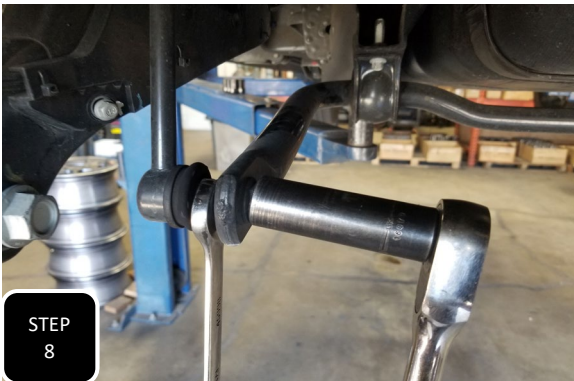
Step 8 Unbolt the sway bar end link from the sway bar on the side you are working on and leave it disconnected.
