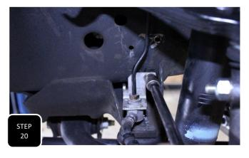
**Step 20** Drill a 1/4" hole, 2 1/8" straight down from the original hole. The factory bolt is self tapping and will thread right in with pressure.
