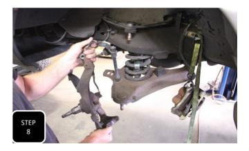
**Step 8** Unbolt the bolt attaching the spindle to the upper ball joint, but do not remove until you have a firm grip on the spindle. Once you do, remove the bolt and then remove the spindle.
