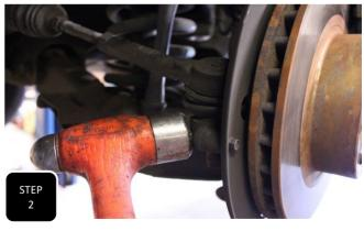
**Step 2** Pull the cotter pin from the castle nut at the tie rod, remove the nut, and then break the rod end loose by hitting the side of the steering arm with a hammer. **NOTE: NEVER HIT THE ROD END ON THE THREADS.**
