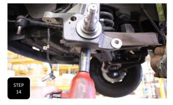
**Step 14** Torque the upper ball joint bolt to 45 ft/lbs and the lower ball joint nut to 120 ft/lbs. For the lower ball joint, further tighten the nut by hand until the opening in the castle nut aligns with the hole in the ball joint and then install the cotter pin.
