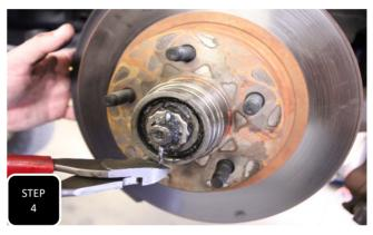
**Step 4** Remove the wheel bearing dust cap to access the wheel bearings. Next, remove the cotter pin from the castle washer and then loosen the nut.
