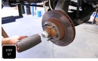
**Step 17** Loosen the nut and then tighten just beyond hand tight. (About 22 in/lbs) Spin the nut a little bit tighter until the opening in the castle nut aligns with the hole in the spindle's spud and then install the provided cotter pin. Next, re-install the dust cap over the wheel bearings using a mallet or dead blow to tap it into place.
