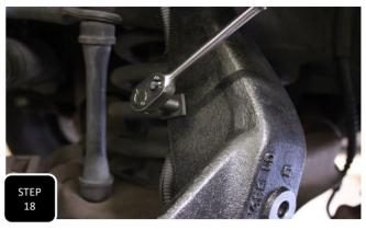
Step 18 Install the ABS sensor using the factory bolt and tighten. Next, attach the ABS wire guide bracket to the side of the spindle using the factory bolt and tighten. NOTE: MAKE SURE TO SPIN THE ROTOR AND CHECK FOR CLEARANCE BETWEEN THE SENSOR AND RELUCTOR RING. IF THERE IS CONTACT, INSTALL A SMALL WASHER BETWEEN THE SENSOR AND SPINDLE. IF THE SENSOR IS WAY TO BIG FOR THE OPENING IN THE SPINDLE THEN YOUR TRUCK HAS STABILITRAC AND THESE SPINDLES WILL NOT WORK.
