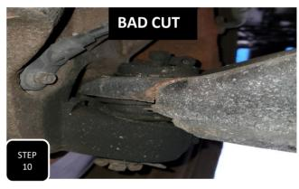
**Step 10** Above is a picture of a good cut and a bad cut. Good cuts are smooth and round off at all transitions. This will prevent the control arm from cracking. When done trimming, spray paint the cut area for rust prevention.
