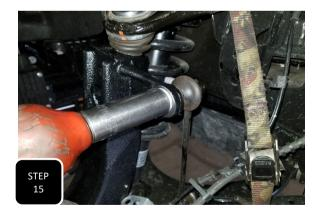
**Step 15** Re-attach the sway bar end link to the neck of the spindle using the factory nut and tighten. **NOTE: THIS SHOULD ONLY BE DONE AFTER BOTH SPINDLES HAVE BEEN INSTALLED.**
