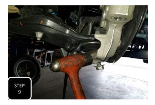
**Step 9** Loosen the nut at the lower ball joint, but do not fully remove it. Next, break the ball joint loose by hitting the side of the spindle, right at the ball joint, with a hammer. The nut will catch the spindle then you can fully remove the spindle. **NOTE: NEVER HIT THE BALL JOINT ON THE THREADS.**
