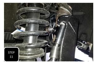
**Step 11** Install the new spindle using the factory ball joint nuts and tighten to factory specs.
