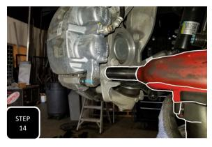
**Step 14** Re-install the brake rotor and then the brake caliper using the factory caliper bolts and tighten to factory specs.
