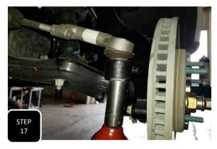
**Step 17** Re-attach the tie rod to the steering arm of the spindle using the facory nut and tighten. Next, repeat steps 1-17 on the other side.
