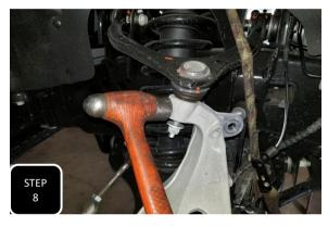
**Step 8** Loosen the nut at the upper ball joint, but do not fully remove it. Next, break the ball joint loose by hitting the side of the spindle, right at the ball joint, with a hammer. The nut will catch the spindle. **NOTE: NEVER HIT THE BALL JOINT ON THE THREADS.**
