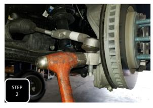
**Step 2** Unbolt the tie rod at the spindle and break it loose by hitting the side of the spindle, right at the joint, with a hammer and separate.
