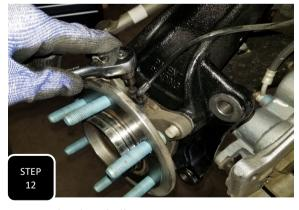
**Step 12** Attach the ABS sensor to the hub assembly using the factory socket head allen screw.
