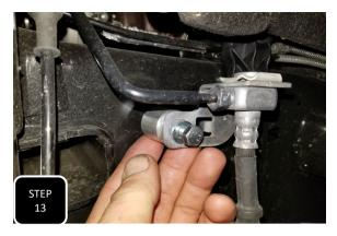
**Step 13** Unbolt the the bracket where the soft brake line meets the hard brake line at the frame and install the provided aluminum spacer with the provided M8-1.25 x 40 bolt then tighten.
