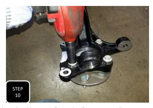
**Step 10** Remove the 4 wheel bearing bolts and then separate the wheel bearing from the factory spindle. Next, attach the wheel bearing to the new spindle using the factory bolts and tighten. **NOTE: THE FACTORY DUST SHIELD WILL NOT GET RE-USED.**
