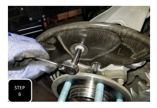
Step 6 Remove the free floating brake rotor and then remove the upper mounting bolt on the dust shield behind it.
