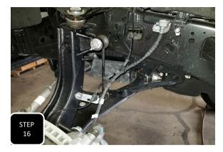
**Step 16** Attach the factory brake line bracket to the neck of the spindle, just above the brake caliper, using the factory bolt and tighten.
