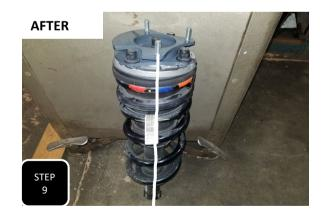
**Step 9** Our spacer will rotate the strut top 55 degrees so the bottom of the shock will need to be rotated to return it to proper alignment with the top.
