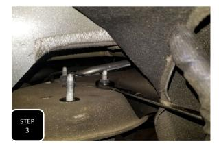
**Step 3** Remove the three nuts attaching the top of the strut to the frame and save for re-installation.
