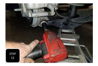
**Step 12** You will need to compress the coil by applying pressure to the lower control arm with a jack until the control arm hole lines up with the spindle hole. Install the factory bolt and tighten to factory specs.
