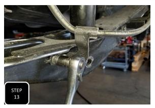
Step 13 Re-attach both brake line guide brackets to the lower control arm and tighten.
