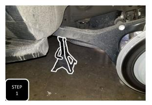
**Step 1** Jack up the rear of the vehicle and support under the frame with jack stands.
