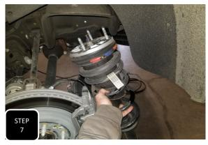
Step 7 Press down on the lower control arm and remove the strut assembly.
