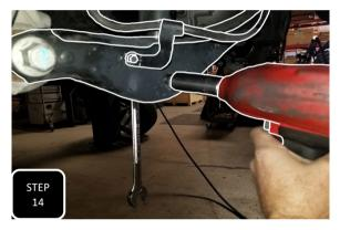
**Step 14** Repeat steps 1-13 on the other side. When both sides have been installed and the truck is back on the ground at ride height, then tighten the lower strut bolt to factory specs.
