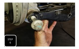
Step 6 Loosen and remove the bolt attaching the lower control arm to the spindle. Save the bolt for re-installation.
