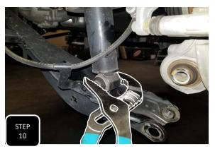
**Step 10** Proper alignment between the top and bottom of the strut can be achieved by compressing the coil and rotating the bottom of the strut. If you do not have a coil compressor, you can attach the top of the strut to the truck and rotate the bottom, using channel locks, until the shock aligns with the control arm.
