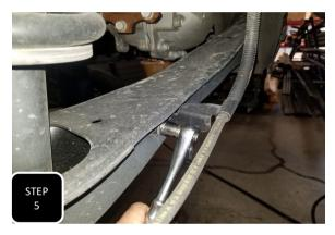
**Step 5** Unbolt both brake line guide brackets from the lower control arm and separate.
