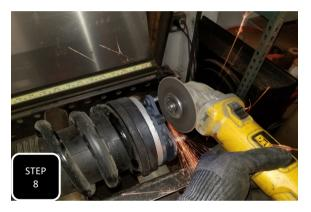
**Step 8** Attach the strut spacer to the top of the strut using the factory nuts and tighten. Next, using a suitable cutting device, cut off the remainder of each factory stud so that they do not stick out higher than the top of the spacer.
