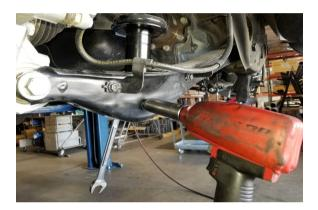
**Step 11** Attach the strut using the provided nuts at the top and the factory bolt at the bottom. You can tighten down the upper nuts, but do not fully tighten the lower bolt until the vehicle is on the ground at ride height.
