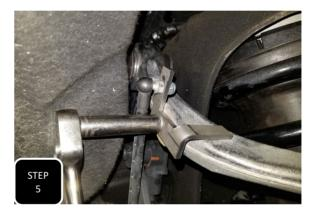
**Step 5** Pop the sensor rod onto the mounting ball using a set of channel lock pliars and squeeze. Next, attach the bracket to the upper control arm using the supplied M6-1.0 x 16 bolt and flat washer. The bent tab needs to sit flat on top of the control arm.
