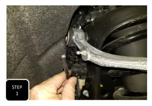
**Step 1** Using a suitable pair of pliars or a flat head screw driver, pry the rod end off of the mounting ball at the front of the upper control arm.
