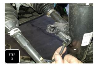
**Step 3** Unplug the wire connection at the body of the front strut and then proceed with installing the strut spacers and then move to step 4.
