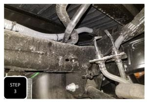
**Step 3** Unbolt the mounting bracket for the brake lines at the frame and separate. **NOTE: THIS WILL ALLOW FOR MORE SLACK IN THE LINES DURING THE INSTALL.**
