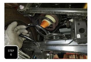
**Step 6** Lower the axle and remove both coil springs along with the bumpstop on top of the coils.
