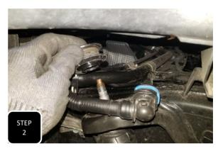
**Step 2** Apply some pressure to the differential with the jack and then unbolt both rear shocks at the frame and remove the upper bushing.
