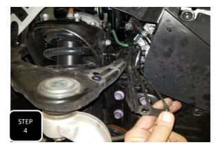
**Step 4** Unbolt the ABS guide bracket from the upper control arm and separate the bracket. **NOTE: THIS WILL ALLOW FOR MORE SLACK IN THE LINE DURING THE INSTALL.**
