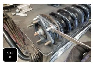
**Step 8** Place the spacer on top of the strut and tighten down using the factory nuts. The 4 bolt pattern is not symetrical and the spacer will align with the part # facing outward.
