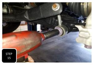
**Step 15** Lower the truck down to the ground and re-install the sway bar end links using the factory hardware. **NOTE: HAVING THE TRUCK ON THE GROUND AT RIDE HEIGHT MAKES INSTALLING THE SWAY BAR ENDS LINKS MUCH EASIER.**
