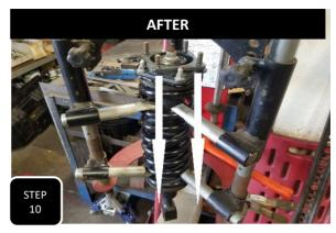
**Step 10** The new strut spacer features a rotated bolt pattern and requires the strut orientation to be rotated in order to align back up with the mounts in the truck. Place the strut assembly in a coil/strut compressor, compress the coil, and rotate the strut so that lower bolt hole is parallel with the part # on the strut spacer top.
