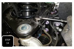
**Step 14** Re-attach both the brake line mounting bracket and the ABS line guide brackets using the factory bolts and tighten.
