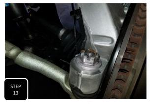
**Step 13** Re-attach the tie rod from the bottom-up, using the factory nut and torque to 60 ft/lbs. Next, re-install the factory cotter pin.
