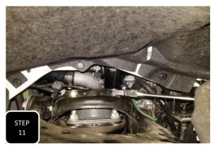
**Step 11** Loosely install the struts lower mounting bolt but do not tighten. Next, attach the top of the strut to the frame using the provided flange nuts and tighten. **NOTE: THE LOWER BOLT WILL GET TIGHTENED WHEN THE TRUCK IS BACK TOGETHER AND SITTING AT RIDE HEIGHT.**
