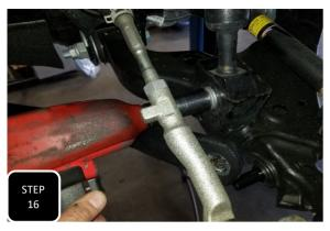
**Step 16** With the truck now on the ground at ride height, torque the lower strut bolts to 80 ft/lbs.
