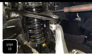
Step 12 Place a floor jack under the lower control arm and jack up a few pumps to get the coil to compress. Next, pull down on the upper control arm and place a pry bar above it to aid in prying down on the UCA while lining up the spindle with the ball joint. Once aligned, attach the UBJ nut and tighten to 80 ft/lbs. NOTE: IT IS POSSIBLE FOR THE AXLE TO POP OUT OF THE CV JOINT WHILE EXTENDED, SO MAKE SURE THE AXLE PROPERLY PLUNGES INTO THE CV BEFORE ATTACHING THE UCA.
