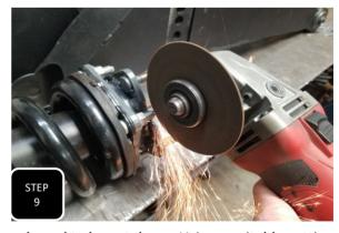
**Step 9** The 4 mounting studs are slightly taller than the spacer and need to be cut down. Using a suitable cutting device, cut each stud down until it is shorter than the top of the spacer.
