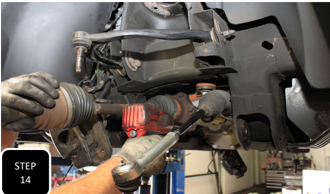
Step 14 Unbolt all 6 bolts attaching the CV axle to the differential housing and remove the axle.
