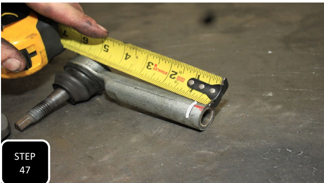
Step 47 Remove the outer tie rod from the inner tie rod and mark a line 1/2" from the end of the threaded hole and cut this 1/2" section off. NOTE: MAKE SURE YOUR CUT IS STRAIGHT SO THAT THE JAM NUT TIGHTENS UP PROPERLY.
