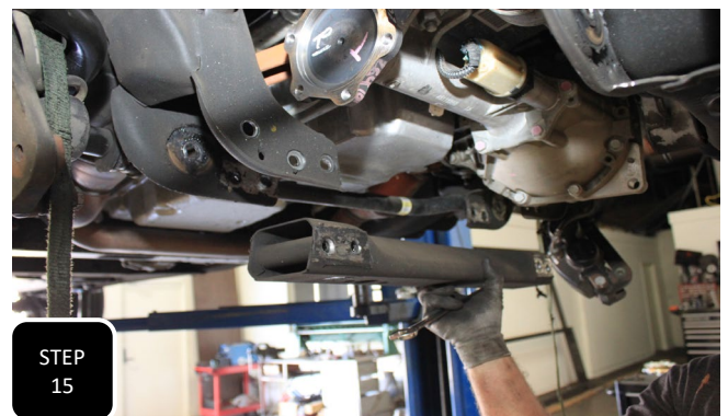
Step 15 Unbolt the 4 bolts attaching the cross member to the rearward lower control arm mount and remove the cross member.
