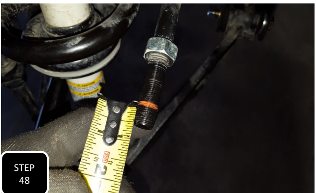
Step 48 Mark a line 9/16" in from the threaded end of the inner tie rod and cut this section off. NOTE: MAKE SURE TO CLEAN UP THE END SO THAT THE OUTER TIE ROD CAN THREAD BACK ON PROPERLY.
