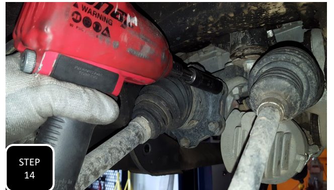
Step 14 Unbolt all 6 bolts attaching the CV axle to the differential housing and remove the axle.
