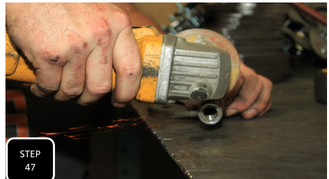
Step 47 Remove the outer tie rod from the inner tie rod and mark a line 1/2" from the end of the threaded hole and cut this 1/2" section off. NOTE: MAKE SURE YOUR CUT IS STRAIGHT SO THAT THE JAM NUT TIGHTENS UP PROPERLY.
