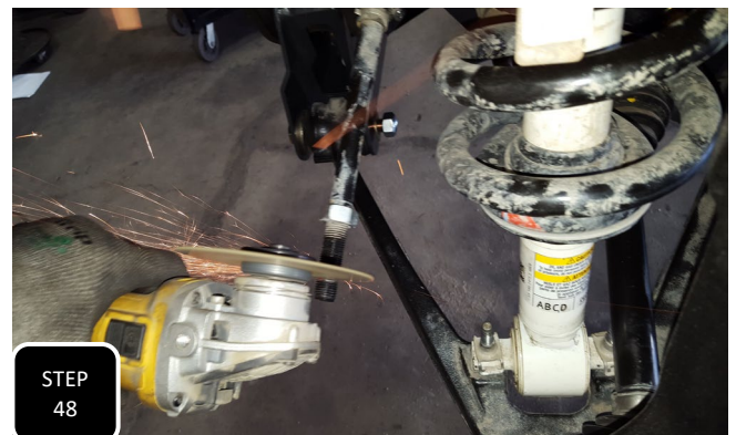
Step 48 Mark a line 9/16" in from the threaded end of the inner tie rod and cut this section off. NOTE: MAKE SURE TO CLEAN UP THE END SO THAT THE OUTER TIE ROD CAN THREAD BACK ON PROPERLY.
