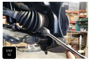
**Step 52** Install the hub assembly into the new steering knuckle using the factory bolts and torque to 120 ft/lbs.
