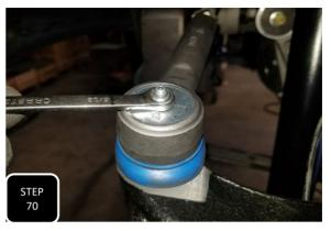
**Step 70** Locate the new, shorter outer tie rod end and thread it onto the inner tie rod end until it is able to connect to the steering knuckle when the steering knuckle is positioned with the rotor parallel to the frame. Next, install the grease fitting and add a little bit of grease to the joint. Lastly, tighten up the rod end to the steering knuckle using the provided nut.
