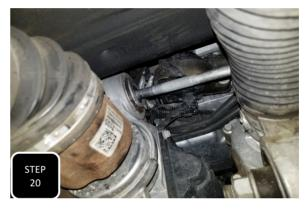
**Step 20** Support the front differential with an adjustable jack and then begin unbolting the mounts. Start with the passenger side mount and remove the long bolt.
