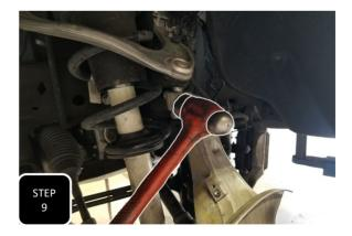
**Step 9** Loosen the upper ball joint nut, but do not remove it. Hit the side of the spindle, right at the ball joint, with a hammer to break it loose. The nut will catch the spindle.
