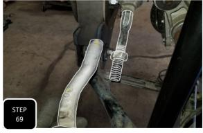
**Step 69** Loosely install the outer tie rod into the steering knuckle to keep the tie rod from rotating while you loosen the jam nut. Break the jam nut loose and then completely unthread and remove the outer tie rod end.
