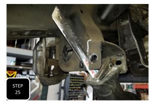
**Step 25** On the front side of this same mount, Scratch a vertical line 2 inches from the edge then on the top side of the mount, connect your two vertical lines. Next, using a suitable cutting device, cut up, across, and down through the middle of your scratched lines.
