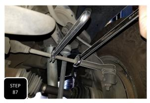
**Step 87** Install the new wheels and tires, then move the truck forward and back about 10 feet while moving the steering back and forth to settle the suspension. Next, adjust the vehicles tow alignment close to straight so that the vehicle is safe to drive to the alignment shop.
