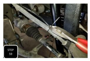
**Step 59** Using two of the provided zip ties, attach the remainder of the ABS line to the brake line and then trim off the tail of the un-used zip tie.
