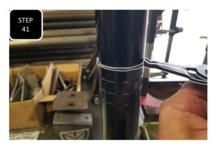
**Step 41** Locate the new lift strut and using a set of retainer ring pliars, install the snap ring into the groove of the desired lift height. The lowest groove is for a 7" lift, the second groove from the bottom is for an 8" lift, the third groove from the bottom is for a 9" lift and the top groove is for a 10" lift.
