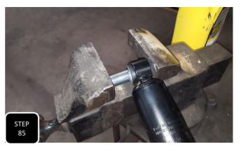
**Step 85** Locate your new longer rear shocks and shock hardware. Next, lube up the bushing on both ends of the shocks and using a bench vise, press the new shock sleeves in. **NOTE: IT HELPS THE PRESSING PROCESS TO PIVOT THE SHOCK UP AND DOWN WHILE CLOSING THE VISE.**
