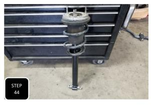
**Step 44** While the stock spring is still compressed, install the new lift strut along with the factory bump stop and tighten using the provided nylock nut. **NOTE: MAKE SURE TO CLOCK THE LOWER BAR PIN THE SAME AS IT WAS WHEN YOU REMOVED THE FACTORY STRUT FROM THE ASSEMBLY.**
