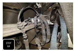
**Step 64** Unclip the brake pad wire from the mount at the upper control arm and then flip the clip up-side down and reinstall it back into the same hole.
