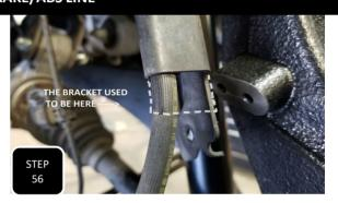
**Step 56** Attach the brake line guide bracket to the side of the spindle using the factory M6 bolt and tighten. Next, pull the brake line down through the mounting bracket to gain some slack between the brake caliper and mounting bracket.
