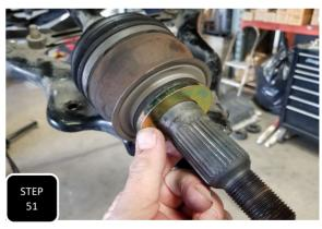
**Step 51** Locate the outer axle spacer which is a 2 3/4" gold washer with a chamfered inner diameter on one side. Slide this down the splined end of the axle with the chamfered end facing inward.
