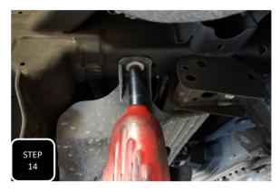
**Step 14** Locate the plastic skid plate between the front bumper and the front suspension then remove and discard it.
