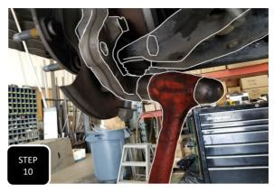
**Step 10** Loosen the lower ball joint nut, but do not remove it. Hit the side of the spindle, right at the ball joint, with a hammer to break it loose. The nut will catch the spindle, then remove the spindle.
