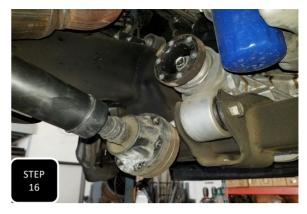
**Step 16** Remove the 6 bolts and connecting plates which attach the front drive shaft to the front differential. Next, support the drive shaft up out of the way.
