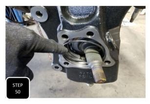
**Step 50** Remove the "O" ring that is in the hub bore of the factory steering knuckle and install it in the new steering knuckle. **NOTE: APPLY SOME WD-40 OR OTHER LUBE ON THE "O" RING TO EASE THE INSTALL OF THE HUB ASSEMBLY.**
