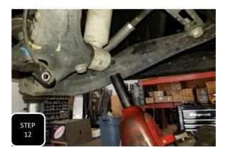
**Step 12** Unbolt the 3 nuts at the top of the strut and the 2 bolts at the bottom of the strut and then remove the strut.
