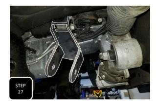
**Step 27** Loosely install the passenger side diff drop bracket using the factory hardware. The bracket needs to swoop towards the front of the truck. **NOTE: DO NOT FULLY TIGHTEN AT THIS TIME.**
