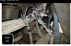
**Step 60** Separate the brake pad sensor wire guide bracket from the brake line guide bracket by detaching where the two brackets clip together. Next, separate the brake pad sensor wire from the bracket at the upper control arm.
