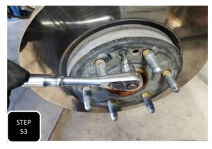
**Step 53** Install the brake rotor onto the wheel studs and secure it using the factory retainer screw.
