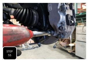
**Step 55** Install the brake caliper using the factory bolts and torque to factory specs.
