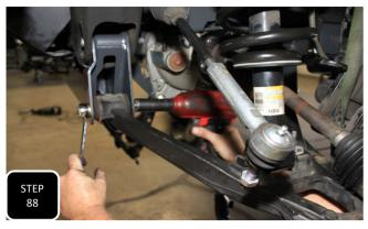
**Step 88** Now that the suspension is settled and the vehicle is sitting at ride height, go back and tighten all of the bolts that were left loose. **NOTE: TIGHTENING THE CONTROL ARM BUSHINGS WHILE THE TRUCK IS AT RIDE HEIGHT WILL PROLONG THE LIFE OF THE BUSHINGS.**
