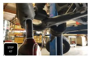
**Step 47** Fully tighten the upper nuts and lower bolts for both struts.
