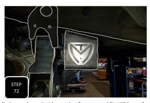
**Step 72** Locate the two sway bar drop down brackets and install them sloped side at the frame and "MT" logo facing outward, using the factory hardware.
