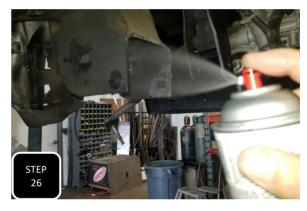
**Step 26** Once you have cut the piece completely off, then clean up any sharp edges, and spray paint for rust prevention.
