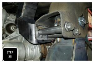
**Step 35** Locate the passenger side diff drop support bracket and loosely install it between the passenger side diff bracket and the frame where the rear cross member was original located. Install the provided sleeves in the gap of the frame and use the factory bolts through the sleeves and into the support bracket. Once all are loosely installed, fully tighten all 3 bolts to 85 ft/lbs.
