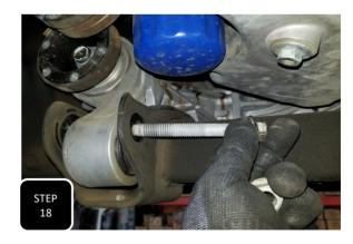
Step 18 Unbolt the diff, just under the yoke to separate it from the cross member
