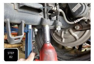
**Step 82** Loosely tighten the U-bolts and then install the lift block and U-bolts on the other side. Once both blocks have been installed, torque the U-bolts to 100 ft/lbs.
