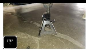
**Step 1** Jack up the front of the truck and support under the frame rails using jack stands.
