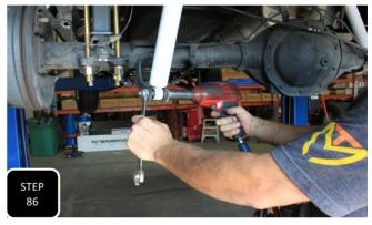
**Step 86** Install the new longer shocks using the factory hardware and tighten. **NOTE: MAX TRAC SHOCKS MUST BE**MOUNTED WITH THE BODY AT THE AXLE AND THE SHAFT AT THE FRAME OR THEY WILL NOT WORK PROPERLY. FOX
