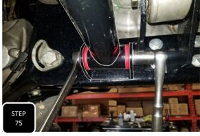
**Step 75** Locate the smaller, clevis looking kicker bar brackets and loosely install them onto the back of the rearward subframe using the supplied 1/2" hardware. Next, loosely install the kickerbars using the supplied 1/2" hardware. Once both kicker bars have been loosely installed, fully tighten both mounts and then lastly tighten all 4 kicker bar bolts. All 1/2" bolts get torqued to 60 ft/lbs and the M18 crossmember bolts to 150 ft/lbs.
