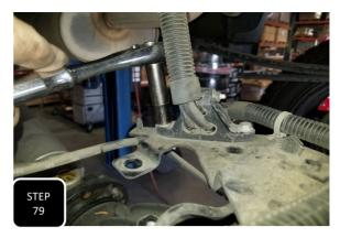
**Step 79** Unbolt the two bolts that attach the ABS wiring to the top of the differntial and allow the wiring to hang loose until the lift blocks are installed.
