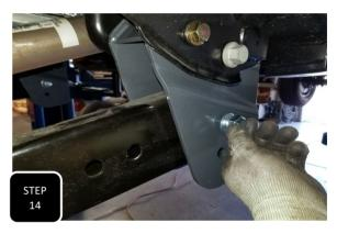
**Step 14** Swing the radius arm up and attach it to the lower hole of the new bracket using the provided M18 bolt, nut, & washers. For a 4" lift attach the arm to the upper of the two holes and for a 6" or 8" lift attach it to the lower of the two holes.
