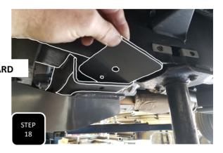
**Step 18** Locate the flat plate labeled DS and slide it into the cross member above the back of the 4 link bracket. Line up the hole and loosely attach the plate and bracket together using the provided M12-1.5 x 40 socket head allen bolt. **NOTE: THE DRIVER'S SIDE IS THE LONGER PLATE**
