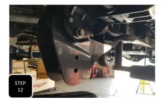
**Step 12** Install the radius arm drop down bracket into the factory radius arm bracket on the frame and loosely attach it using the factory bolt at the big hole and the provided  $3/8-16 \times 41/2$ " bolt at the small hole.
