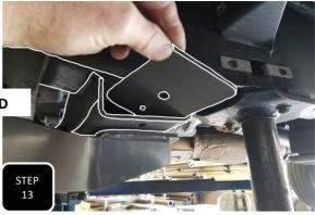
**Step 13** Locate the flat plate labeled DS and slide it into the cross member above the back of the radius arm bracket. Line up the hole and loosely attach the plate and bracket together using the provided M12-1.5 X 40 socket head allen bolt. **NOTE: THE DRIVER'S SIDE IS THE LONGER OF THE TWO PLATES.**
