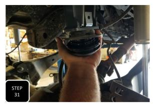
**Step 31** Attach the factory bump stop mounting cup to the bottom of the drop down bracket using the provided M8 bolt, nut, and washers. Once tight, then pop the factory bump stop back in. On the driver's side, you will attach the provided Vacuum line mounting bracket as pictured. **NOTE: SPRAY THE BUMPS STOP WITH WD-40 TO EASE THE INSTALL PROCESS.**
