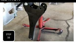
**Step 16** Loosen all 3 radius arm mounting bolts, 2 at the axle and 1 at the frame and then remove the radius arm. **NOTE: WORK ON ONE SIDE AT A TIME SO THAT THE AXLE IS SAFELY SUPPORTED AT ALL TIMES.**
