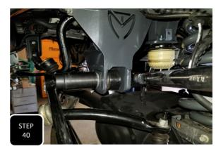
**Step 40** When attaching the trac bar to the drop down bracket, you will need to use the provided off-set plates. The hole will need to be off-set to the driver's side for the 4" lift or towards the passenger side for the 8" lift. Use the factory M18 bolt and nut and only loosely attach for now. **NOTE: THE TRAC BAR WILL GET FULLY TIGHTENED WHEN THE TRUCK IS ON THE GROUND AT RIDE HEIGHT.**
