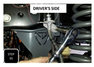
**Step 35** You will need to gently unravel the factory, hard brake line so that the soft line now points downward and the factory mounting bracket lines up with the two holed flange on the provided mounting bracket. Next, attach the factory bracket to the provided bracket using the provided M8 bolt, nut, and washers.
