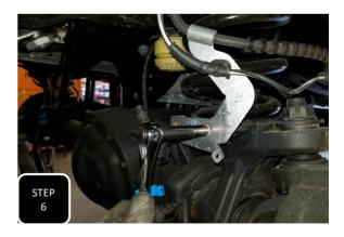
**Step 6** Unbolt the brake line brackets at the frame and at the axle to allow for slack when lowering the axle.
