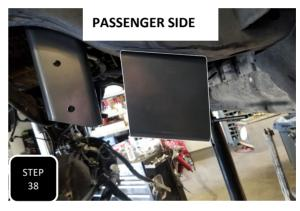
**Step 38** Intstall the new sway bar drop down brackets. You will notice that one of the vertical sides has more angle to it than the other. The more angled side will face the rear of the truck and open end of the bracket will face toward the middle of the truck. Attach each side to the frame using the factory nuts and tighten.
