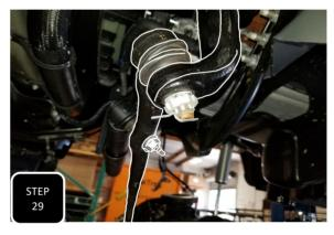
**Step 29** Attach the drag link to the pitman arm, from the top down, using the factory nut and tighten. Next, install the castle sleeve and the factory cotter pin.
