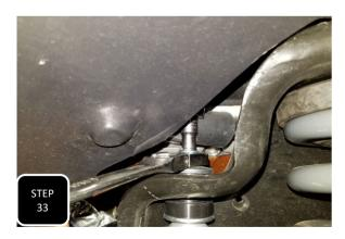
**Step 33** Tighten up both ends of both front shocks.
