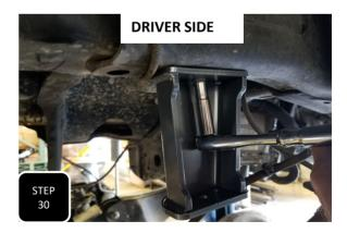
**Step 30** Pop the factory bump stop out of its mounting cup then unbolt the cup and using the same bolt, attach the new bump stop drop down bracket to the same mounting hole. The angled side of the bracket will face the rear of the truck, the shorter of the two surfaces downward, and the open end outward.
