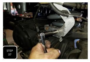
Step 37 Using the factory bolt, re-attach the brake line bracket to the lower coil mount as it was originally.
