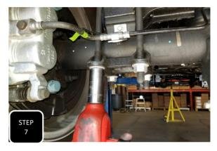
**Step 7** Once cut to length, install the U-bolts with the factory U-bolt plate and snug down. You will want to then loosen the U-bolts on the other side to allow the axle to rotate, and then fully tighten and torque the U-bolts to 140 ft/lbs. Next, install the block on the other side and torque down the U-bolts.
