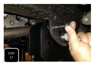
**Step 17** Loosely install the 4 link bracket using the factory M18 bolt at the large hole and the provided 3/8-16 x 4 1/2" bolt at the small hole.
