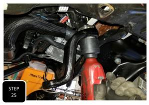
**Step 25** Apply a conservative amount of thread locker to the threads of the factory nut then attach the new drop down pitman arm to the steering box using the factory nut. Once tight, then torque to 350 ft/lbs. **NOTE: MAKE SURE TO INSTALL THE NEW PITMAN ARM IN THE EXACT SAME DIRECTION AS THE OLD ONE CAME OFF.**
