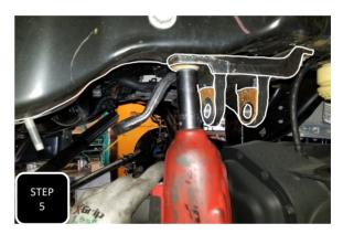
**Step 5** Unbolt all 5 mounting bolts for the trac bar bracket on the frame and remove the bracket.
