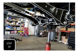
**Step 10** Once both sides have the coils removed and are supported by the new shocks, move the adjustable jack to the middle of the axle and apply pressure.
