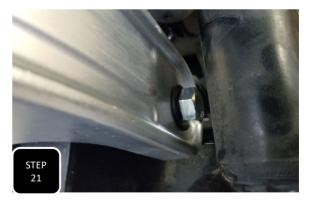
**Step 21** Insert the larger machined sleeves into the upper link arm hole at the axle side of the link. Both sleeves get installed from the outside facing inward then attach the link to the axle using the provided M18 bolt, nut and washers.
