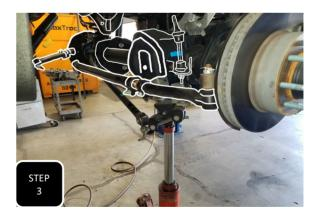
**Step 3** Unbolt the trac bar from the bracket on the frame and separate.
