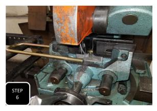
**Step 6** Depending on what leaf pack is in your truck, the U-bolts included in this kit may need to be cut down. If this is the case, install them, measure how much you want to cut off, and then do so for the cleanest install possible.
