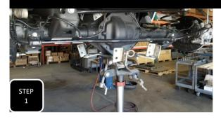
**Step 1** Jack up the rear of the truck and support under the frame rails with jack stands. **NOTE: KEEP AN ADJUSTABLE JACK UNDER THE AXLE FOR HEIGHT ADJUSTMENT.**
