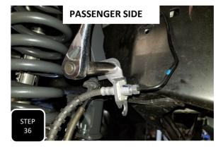
**Step 36** The passenger side ABS/ brake line bracket will mount the same as the driver's side and also require the unraveling of the factory hard brake line to line up with the new bracket.
