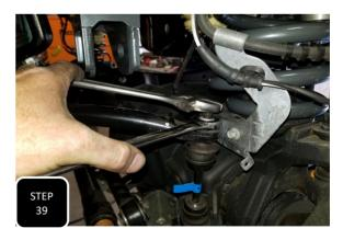
**Step 39** Attach the sway bar to the drop down brackets using the provided M10 bolts, nuts, and washers then tighten. Next, re-attach the ends to the end links on the axle using the factory nuts and tighten.
