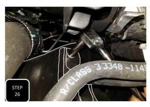
**Step 26** Remove the two mounting bolts that attach the factory steering stabilizer bracket to the passenger side frame and separate.
