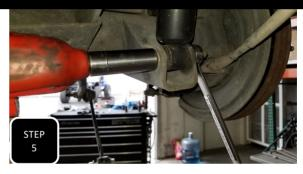
Step 5 Install the new shocks and tighten using factory hardware at the bottom. NOTE: MAXTRAC SHOCKS ARE A TWIN TUBE SHOCK THAT NEEDS TO BE FULLY CYCLED BEFORE INSTALL SO FULLY COMPRESS THEM & LET THEM REBOUND ABOUT 2-3 TIMES.
