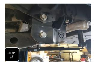
**Step 18** Loosely install the radius arm using the factory bolts at the axle and the provided M18 x 130 bolt at the bracket. **NOTE: DO NOT FULLY TIGHTEN ANY OF THESE 3 BOLTS UNTIL THE TRUCK IS ON THE GROUND AT RIDE HEIGHT.**
