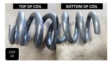
**Step 34** Place the rubber isolator on top of the new coil and install the coil. Make sure the nipple on the isolator aligns with the hole in the coil bucket then jack up the axle so that pressure is applied and re-attach the shock. **NOTE: THE COIL NEEDS TO BE INSTALLED WITH THE FLATTER SIDE FACING UPWARD AND THE PART # RIGHT SIDE UP.**
