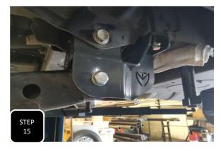
**Step 15** Loosely install the radius arm using the factory bolts at the axle and the provided M18 x 130 bolt at the bracket. **NOTE: DO NOT FULLY TIGHTEN ANY OF THESE 3 BOLTS UNTIL THE TRUCK IS ON THE GROUND AT RIDE HEIGHT.**
