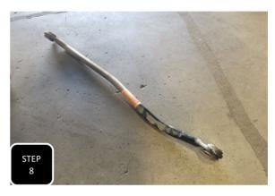
**Step 8** Unbolt the trac bar from the axle and completely remove the trac bar. Save the hardware for re-installation.
