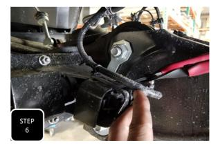
**Step 6** Unbolt the brake line bracket on both axles and unclip the wiring harness for the 4wd module. **NOTE: THIS IS A SAFETY PRECAUTION SO AS NOT TO DAMAGE EITHER DURING THE INSTALL.**
