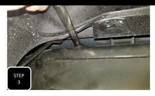
**Step 3** The top of the shock on Ram 2500's is a standard stem that is hidden behind the plastic wheel well liner. Using a knife, cut a clean opening for access to the stem nut and remove the shock.
