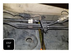
**Step 32** Use the supplied zip tie to attach the fuel line assembly to the U-bolt.
