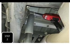
**Step 2** The top of the shock on Ram 3500's is a standard loop with a bushing. Remove the nut and then the shock.
