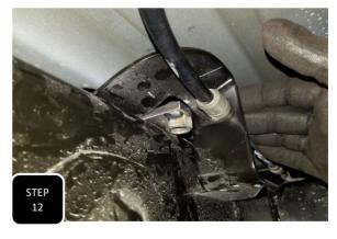
**Step 12** Insert the provided 9428RAB-2 nut plate on top of the frame, behind the E-brake bracket with the notched edge facing the front of the truck and the nut towards the outside of the frame facing downward. **NOTE: THIS E-BRAKE BRACKET IS ONLY ON 2021 AND NEWER TRUCKS.**
