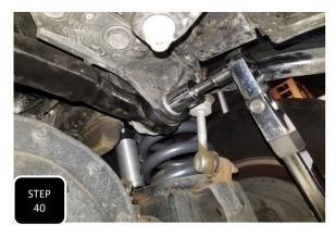
**Step 40** Torque both trac bar mounting bolts to 250 ft/lbs.
