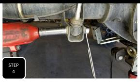
**Step 4** Install the new shocks and tighten using factory hardware. Max Trac shocks need to be installed with the shaft of the shock at the frame and the body at the axle. Fox shocks get installed opposite of that. **NOTE: MAXTRAC SHOCKS ARE A TWIN TUBE SHOCK THAT NEEDS TO BE FULLY CYCLED BEFORE INSTALL SO FULLY COMPRESS THEM & LET THEM REBOUND ABOUT 2-3 TIMES.**
