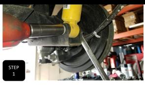
**Step 1** Jack up the rear of the truck and support under the frame with jack stands. Apply pressure to the rear diff with an adjustable jack and remove both rear shocks.
