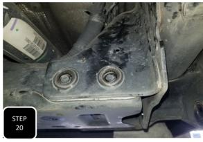
**Step 20** Remove the mounting nuts for the cross member just inside the radius arm bracket and push the bolts back so that the heads are not sticking out of the cross member.
