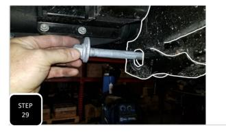
**Step 29** Loosely attach the links to the axle using the provided M18 bolts. After the first link is attached, you will want to remove one of the radius arm bolts, at the axle, on the other side so that the axle can be slightly rotated to attach the second link.
