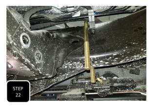
**Step 22** Working at the front of the cross member, pry the plastic fuel line guide bracket away from the frame and install the provided U-bolt over the frame from the top down with the shorter leg of the U-bolt on the inside of the frame.
