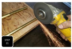
**Step 21** Locate the provided 9" long, square U-bolts for the 4link brackets, mark a cut line 1/2" down the threads of "only" one side, then cut that leg off the U-bolt on that line so that it is 1/2" shorter.
