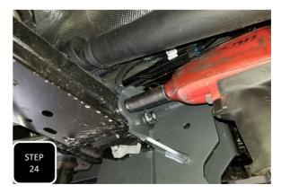
**Step 24** First snug up the U-bolt nuts, then the cross member bolts, and lastly the original radius arm bolt. Once all is snug and the bracket is up in place, go back and torque all bolts to factory specs. The U-bolt should get torqued to 100 ft/lbs.
