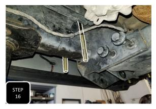
**Step 16** For the passenger side, slide the supplied U-bolt over the frame, just behind the cross member behind the factory radius arm bracket and allow it to hang vertically.
