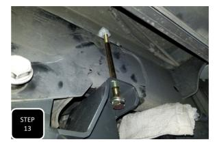
**Step 13** Models without the welded on brake line will look like this to where the nut plate will openly sit on top of the frame.
