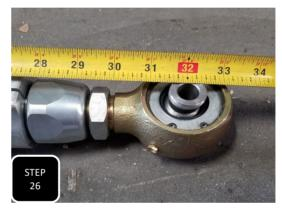
**Step 26** Adjust the upper links to 28.5" (the shorter link) and the lower links to 31 5/8" (the longer link). Now locate the links for the side that you are working on first. The driver's side links, when installed will have the Max Trac logo facing upright and the two pinch bolts facing outward when installed. **NOTE: THE LENGTH OF THE ARMS IS MEASURED FROM CENTER OF MOUNTING HOLE.**
