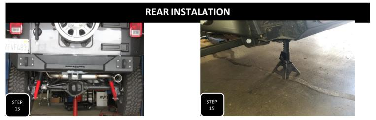
**Step 15** Jack up the rear of the truck and support under the frame with jack stands. Keep an adjustable jack under the differential for height adjustment.
