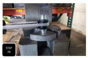
**Step 26** Locate the new rear shocks and press in the provided hardware. The top hardware consists of two sleeves with a rib in the middle and the bottom sleeve is just a straight sleeve. First grease the bushings and then press in the sleeves using a bench vise or arbor press.
