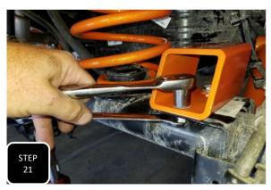
**Step 21** Attach the new bump stop extensions to the axle using the provided 3/8" hardware. The extensions will need to off-set towards the front of the truck.
