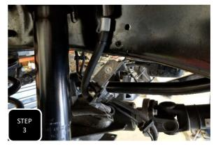
Step 3 Unbolt both front brake line brackets from the frame and pull the bracket away from the frame.
