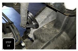
**Step 14** Re-attach both wire clips for the front differential wiring and then move to the rear of the vehicle.
