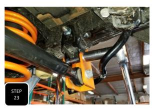
**Step 23** Install the supplied  $1/2 \ge 5 1/2$ " bolt through the side of the bracket/frame and torque to 85 ft/lbs. Next, loosely attach the trac bar to the new bracket using the factory hardware, but do not tighten at this time. Tighten the bolt through the original trac bar hole and torque to 100 ft/lbs.
