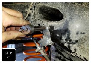
**Step 25** Locate the brake line extension brackets and attach them with the bent tab facing down, inward, and towards the front of the truck. Loosely install them using the factory mounting bolt. Next, attach the factory bracket to this bracket using the provided 1/4" hardware. Rock both brackets forward so the tab on the new bracket hits the frame and the tab on the factory bracket hits the new bracket and tighten both bolts.
