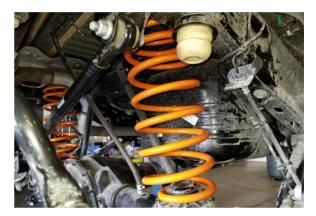
**Step 20** Install the new coil spacers on the lower coil mount and then re-install the plastic isolator. Next, install the new springs and jack up the axle until both springs are properly seated.
