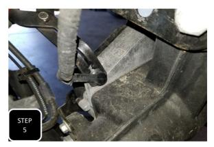
**Step 5** Before lowering the front axle, release the two wire guide clips for the front differential wiring so that the wiring does not get damaged during the install.
