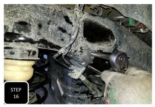
**Step 16** Working on both sides at the same time, unbolt the brake line guide bracket from the frame and pull down the hard line a little bit to gain slack in the line.
