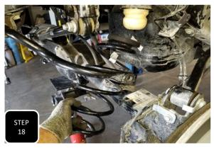
**Step 18** Lower down the axle and remove both coil springs.
