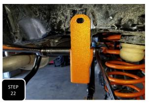
**Step 22** Unbolt the trac bar from the mount at the frame and separate. Loosely attach the new trac bar bracket using the supplied M14 hardware and zinc plated crush tube. The new bracket will fit around the factory bracket.
