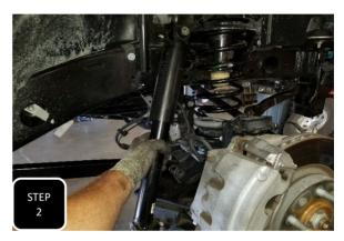
**Step 2** Working on both sides at the same time, apply some pressure on the axle with the floor jack centered under the front axle and then unbolt both front shocks at both ends and remove.
