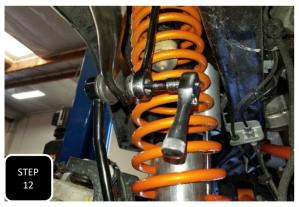
**Step 12** Install the factory rear sway bar end links on the front using the factory hardware.
