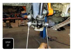
**Step 27** Once the mounting hardware has been installed, install the shocks on the truck using the factory bolts top and bottom. Torque bolts to 55 ft/lbs.
