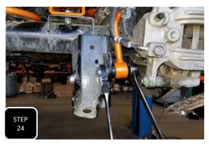
**Step 24** Attach the new sway bar end links to the sway bar using the supplied M12 hardware and to the axle using the factory M12 hardware. The links will need to go wider at the sway bar. Next, torque the bolts to 50 ft/lbs.
