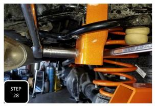
**Step 28** Install the wheels and tires then lower the truck down to ride height. Jump on the rear bumper a few times to settle the rear suspension then torque the trac bar bolt to 100 ft/lbs.
