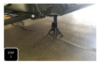
**Step 1** Jack up the front of the vehicle and support under the frame with jack stands. Keep an adjustable jack under the axle for height adjustment.
