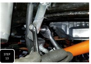
**Step 13** Locate the brake line extension brackets and loosely attach them to the frame using the factory bolts. The bent tab will face out, away from the frame. Next, attach the two brackets together using the provided 1/4' hardware and rotate the brackets until the bent tab on the factory bracket touches the new bracket, and tighen. Lastly, tighten the bolt at the frame.
