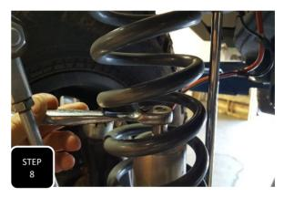
**Step 8** Drop the supplied 7/16" bolt and washer into the bumpstop and tighten down to 45 ft/lbs.
