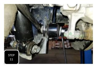
**Step 11** Your factory rear sway bar end links will get used in the front so now proceed to the rear of the truck and remove both factory sway bar end links.
