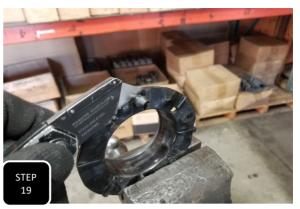
**Step 19** Remove the plastic lower coil isolator and cut off the guide nipple using a suitable cutting device.
