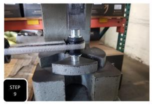
**Step 9** Locate the new front shocks and press in the provided hardware. The top hardware consists of two sleeves with a rib in the middle and the bottom sleeve is just a straight sleeve. First grease the bushings and then press in the sleeves using a bench vise or arbor press.
