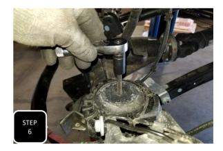
Step 6 Lower the axle and remove both front coil springs. Next, using a 7/16-14 tap, thread the center hole in the coil guide on the axle.
