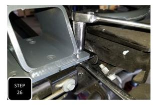
**Step 26** Install both rear bump stop extensions using the provided M8 bolts, nuts, and washers. Install the the extension with the square tube angling forward on the vehicle.
