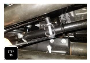
**Step 30** Using a tape measure, find a consistant spot to measure the distance between the inside of each front tire to the frame. Loosen the clamps on the adjustable front trac bar and adjust the length of the trac bar until you read the same measurement on both sides. The tighten down the clamps.
