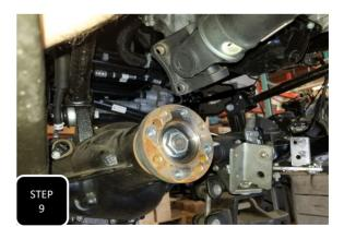
**Step 9** Remove all four of the front drive shaft mounting bolts at the differencial and separate the drive shaft from the drive flange. Support the drive shaft up out of the way.
