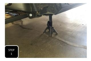
**Step 1** Jack up the front of the vehicle and support under the frame rails with jack stands. Leave an adjustable jack under the middle of the axle and apply some pressure.
