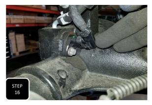
**Step 16** Unclip the wire guide for the front diff plug from the inside of the frame near the steering box. This will allow for more slack in the line and you can now re-attach the plug to the diff.
