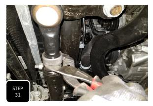
**Step 31** Position the front tires until they are evenly facing forward. Loosen the tension clamp on the drag link and adjust it until the steering wheel is straight again, then tighten the tension clamp back down.
