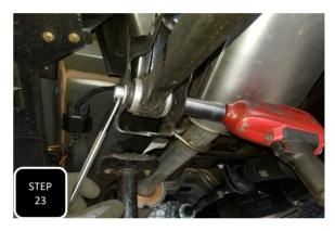
**Step 23** Loosen all 4 control arm mounting bolts enough to take tension off of the bushings. This will allow for an easier install of the new coils.
