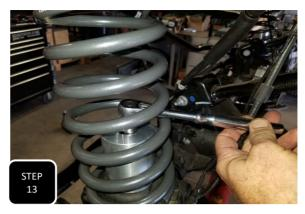
**Step 13** Locate the front bump stop extensions and hold them right side up, inside the new coil, while installing the new coils. Once the coils are seated, attach the bump stop extensions using the provided 7/16-14 x 2 1/2" bolt and washer, then tighten.
