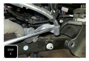
**Step 5** Once cut, use a screw driver to pry open the wrap around the line and remove the bracket.
