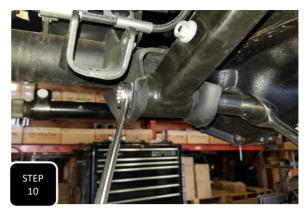
**Step 10** Loosen all four bolts that attach each of the control arms to the front axle, but do not remove. **NOTE: THIS WILL ALLOW FOR THE AXLE TO DROP LOWER AND MAKE IT EASIER TO INSTALL THE NEW COILS.**
