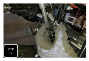
Step 17 Re-attach all other wire guides that were disconnected during the disassembly process.
