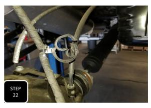
**Step 22** Unbolt both rear brake line brackets at the frame and then separate the clip the attaches the rear diff wiring to the e-brake cable near the diff.
