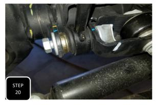
**Step 20** Install the rear sway bar end links in the front of the vehicle using the factory hardware. You will need to use the provided thick and thin gold washers to allow for a snug fit on the passenger side axle mount.
