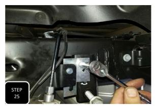
**Step 25** Attach the provided rear brake line brackets to the factory brake line bracket using the provided M6 bolt, nut, and washer. Then attach the bracket to the original brake line mounting hole using the factory bolt and tighten. **NOTE: THE BRACKETS ARE SIDE SPECIFIC SO AND WILL ONLY FIT ONE WAY.**
