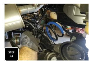
**Step 24** Lower the axle and remove both coils. Transfer over the rubber isolator to the new coils and install them both into the vehicle.
