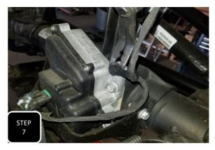
**Step 7** Separate the wire guide from the passenger side upper control arm and then from the motor housing on the axle to allow for more slack when removing the coils.
