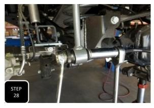
**Step 28** Install the new rear sway bar end links using the factory bolt at the frame and the provided M12 bolt, nut, and washers at the sway bar. **NOTE: THERE IS A NARROW BUSHING AND A WIDER BUSHING ON THESE END LINKS. MAKE SURE THE NARROW BUSHING GETS ATTACHED AT THE FRAME.**
