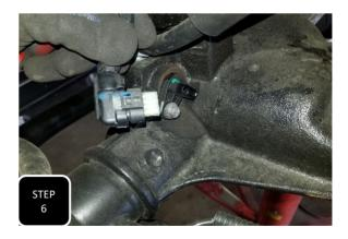
**Step 6** Un-clip the diff plug wire guide from the driver's side upper control arm clevis and then separate the plug from the diff. This will prevent the wire from getting damaged when removing the coils.
