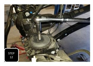
**Step 12** Before installing the new coils, you will need to thread the hole in the coil seat on the axle using a 7/16-14 tap.
