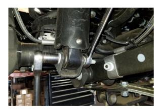
**Step 3** Unbolt both front shocks from the axle only and separate.
