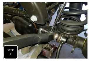
Step 2 Unbolt both front sway bar end links from both ends and remove. NOTE: THEY WILL NOT BE RE-INSTALLED.
