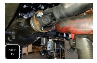
**Step 15** Re-attach the drive shaft to the front diff using the factory bolts and tighten.
