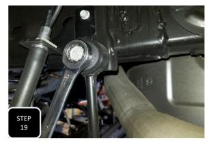
**Step 19** Go to the rear of the vehicle and remove the factory sway bar end links. They will now be utilized in the front.
