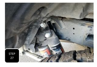
**Step 27** Attach the shock extender to the shock using the supplied bolt and then to the frame using the facotry bolt. The shock extenders are identicle so they can go on either side. Torque bolts to 90 ft/lbs.
