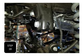
**Step 18** Loosely attach the new adjustable front trac bar using the factory hardware. **NOTE: DO NOT WORRY ABOUT FULLY TIGHTENING OR ADJUSTING THE TRAC BAR UNTIL THE VEHICLE IS BACK ON THE GROUND AT RIDE HEIGHT.**
