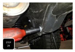
**Step 29** Install the wheels and tires and then lower the truck down so it is now on the ground at ride height. Fully tighten all of the control arms that you loosened and the front trac bar at both ends.
