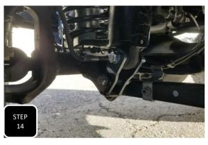
**Step 14** Install the front shock extenders using the factory bolt at the axle and provided bolt at the shock. These extenders are bent opposite of each other, but can fit on either side. Torque bolts to 90 ft/lbs. **NOTE: IT IS RECOMMENDED TO HAVE THE ANGLED SIDE OF THE EXTENDER FACING THE FRONT OF THE TRUCK AND THE STRAIGHT SIDE FACING THE REAR.**
