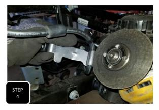
**Step 4** Unbolt the front brake line guide bracket at both lower control arms. Using a suitable cutting device, cut a line about half way into where the bracket wraps the brake line to create a weak spot. **NOTE: BE VERY CAUTIOUS NOT TO NICK OR CUT THE LINE.**
