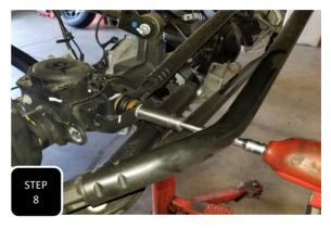
Step 8 Unbolt the front trac bar from both ends and remove. NOTE: THE FRONT TRAC BAR WILL NOT GET RE-USED.
