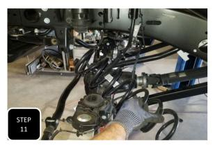
**Step 11** Lower the front axle down and remove both front coils.
