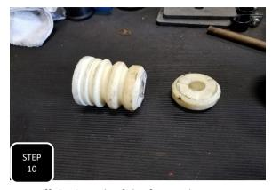
**Step 10** If installing the strut at the 3 drop level, you will need to trim off the last rib of the factory bump stop.
