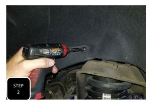
**Step 2** Remove the two torx head bolts that attach the wheel well skirt to allow easier access to the top of the strut.
