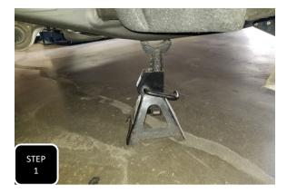
**Step 1** Jack up the rear of the vehicle and support under the frame with jack stands.
