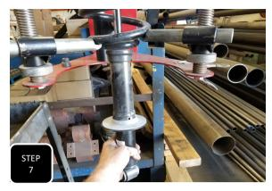
**Step 7** Remove the strut from the vehicle, place it in a strut compressor to compress the coil and remove the middle nut at the top of the strut. Next, remove the factory shock from the strut assembly. **NOTE: TAKE NOTE OF THE POSITION OF THE TOP THREE STUDS IN RELATION TO THE LOWER SLEEVE. THIS WILL HELP WITH RE-ASSEMBLY.**
