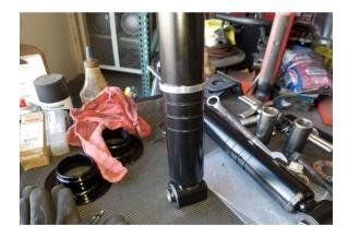
**Step 9** Slide the retainer clip collar down over the retainer clip. Make sure that it slides completely over the clip and rests down on the inside, machined lip then install the lower coil seat over that.
