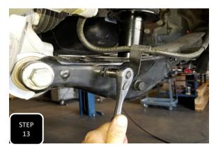
**Step 13** Re-install the control arm bolt at the spindle and tighten to factory specs. Next, re-attach the brake line bracket using the factory bolt and tighten.
