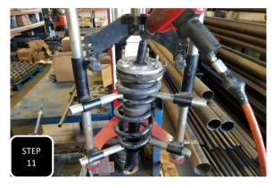
**Step 11** Install the new strut into the coil along with the factory bump stop and tighten using the provided nylock nut. **NOTE: ENSURE THAT THE TOP THREE STUDS ARE POSITIONED IN THE CORRECT ORIENTATION IN RELATION TO THE BOTTOM SLEEVE.**
