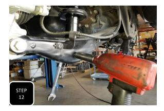
**Step 12** Re-install the strut back onto the vehicle using the factory hardware. You can tighten down the upper nuts, but do not fully tighten the lower bolt until the vehicle is on the ground at ride height.
