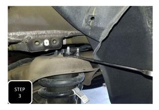
**Step 3** Remove the three nuts attaching the top of the strut to the frame and save for re-installation.
