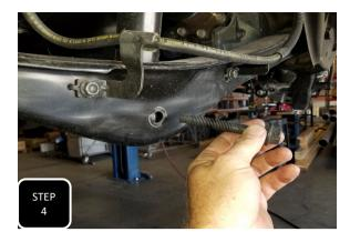
**Step 4** Loosen and remove the lower strut mounting bolt and save for re-installation.
