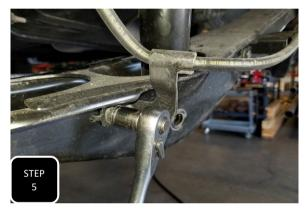
**Step 5** Unbolt the brake line guide bracket from the lower control arm and separate.
