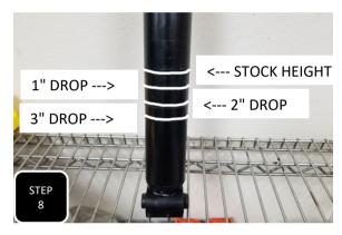
**Step 8** Locate the new lowering strut and set the retainer clip in the appropriate groove for the amount of drop that you are looking to achieve. The top groove is stock, next down is 1" drop, then 2" drop, and 3" drop.
