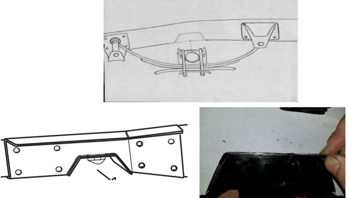
**Step 3** Mark the area that needs to be cut out. This can be achieved by either measuring the "C" area of the fame support and drawing that onto the frame with your center mark at the center of your cut out or by making a template of the frame support and tracing that onto the frame.
