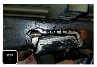
Step 4 Cut out the scribed line using a plasma cutter or other suitable cutting device
