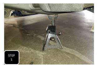
**Step 1** Jack up the rear of your vehicle and support under the frame with jack stands. Allow the suspension to extend to full droop and remove the wheels. **NOTE: IT IS RECOMMENDED TO INSTALL THE FLIP KIT FIRST SO THAT YOU CAN MARK WHERE THE CENTER OF THE AXLE WILL CONTACT THE FRAME.**
