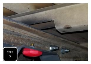
**Step 5** Before being able to test fit the frame support, you may need to trim the bed rib, directly above, if your truck is equipped with one. Using a suitable cutting device, trim the bed rib about 1/2" up from the bottom. Trim from the end of the rib to at least the inside edge of the frame to ensure an easy install of the frame support and no contact of the two.
