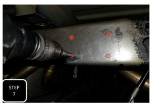
**Step 7** Using clamps, attach the frame support to the frame and mark the holes using a marker or transfer punch. You can even just use the frame support as a guide if that is easiest for you. Next, drill a 9/16" hole through everyone of your marks.
