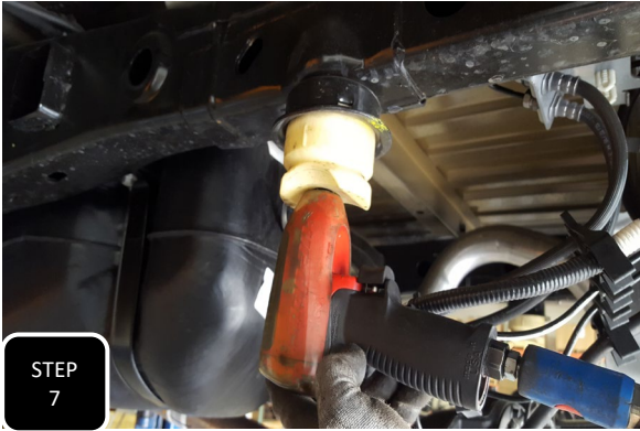
Step 7 Remove both rear bump stops from the frame.
