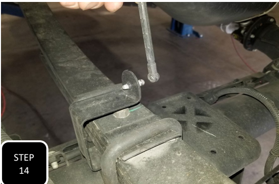
Step 14 Once the lowering shackles have been installed then re-attach the sensor rod to the factory mounting plate at the axle.
