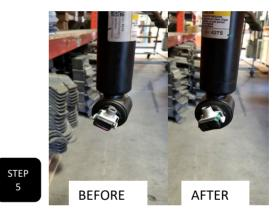
**Step 5** Using an automotive coil/strut compressor, compress the coil so that the bottom of the strut can be rotated 180 degrees. NOTE: THE LOWER BAR PIN IS VULCANIZED AT AN ANGLE AND NEEDS TO BE ROTATED TO ANGLE IT IN THE PROPER DIRECTION AFTER INSTALLING THE STRUT SPACER.
