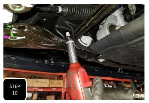
**Step 10** Tighten the nuts at the top of the strut spacer then re-attach the lower control arm cross brace.
