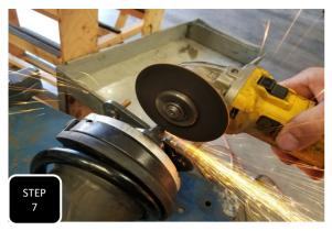
**Step 7** Using a suitable cutting device, cut down the factory studs so that they are not taller than the top of the spacer.
