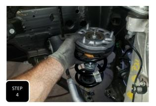
**Step 4** Unbolt both of the bolts attaching the lower control arm cross brace to the lower control arm and remove. Next, remove the strut assembly through the opening in the lower control arm.
