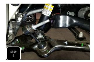
**Step 2** Remove the nut attaching the sway bar end link to the sway bar and separate the two.
