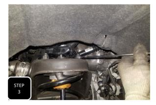
Step 3 Unbolt the two mounting bolts at the bottom of the strut along with the three nuts at the top of the strut.
