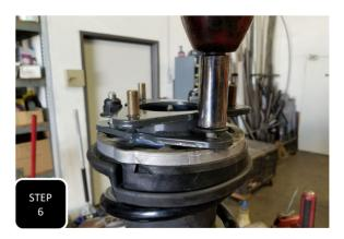
**Step 6** Install the new strut spacer and attach using the factory strut top hardware.
