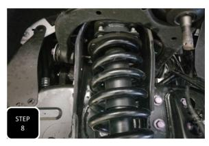
**Step 8** Place the spacer on top of the strut and tighten down using the factory nuts. The 4 bolt pattern is not symetrical and the spacer will align with the part # facing outward. Next, re-install the strut assembly. **NOTE: SINCE THE STRUT ASSEMBLY IS NOW TALLER, IT WILL BE MORE DIFFICULT TO INSTALL AND REQUIRE PUSHING THE LOWER CONTROL ARM DOWNWARD TO CLEAR THE LOWER MOUNTING BOX.**
