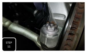
**Step 11** Re-attach the tie rod from the bottom-up, using the factory nut and torque to 60 ft/lbs. Next, re-install the factory cotter pin.
