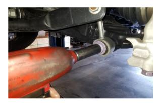
**Step 14** Lower the truck down to the ground and re-install the sway bar end links using the factory hardware. **NOTE:** HAVING THE TRUCK ON THE GROUND AT RIDE HEIGHT MAKES INSTALLING THE SWAY BAR ENDS LINKS MUCH EASIER.
