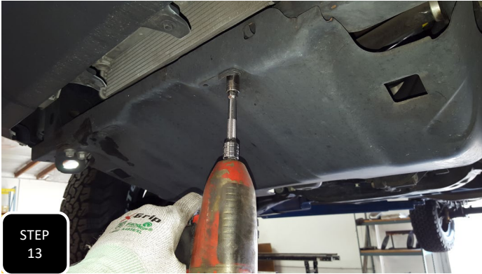
Step 13 Unbolt all 4 bolts holding the primary skid plate on and remove the skid plate.
