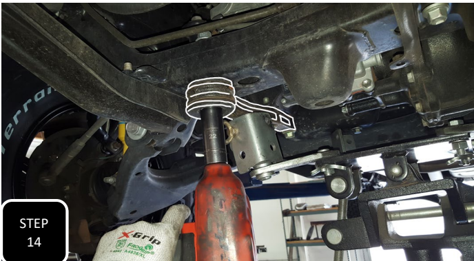
Step 14 Place an adjustable jack under the front differential and remove the two front mounting bolts. NOTE: THERE IS ONE MORE DIFF MOUNT TOWARDS THE BACK ON THE DRIVER'S SIDE THAT THE DIFF WILL PIVOT DOWNWARD ON.
